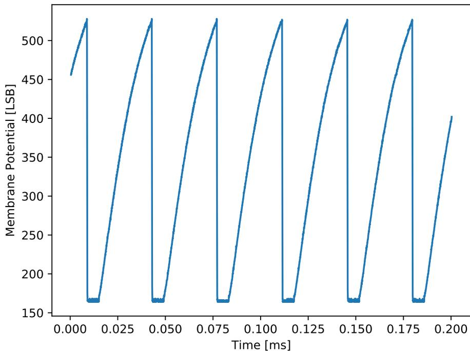
Figure 3: Membrane Potential of a Leak over Threshold Neuron
