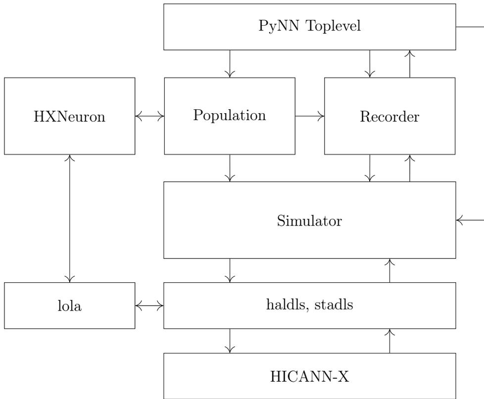
Figure 2: Schematic of the underlying PyNN Structure
