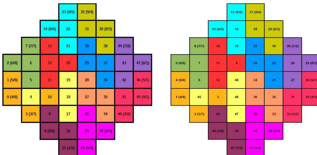
Figure 3: DNC numbers on the left and reticle numbers on the right. The (x/y) at the borders are array coordinates. The wafer is turned around 45 degrees below the bracket.
