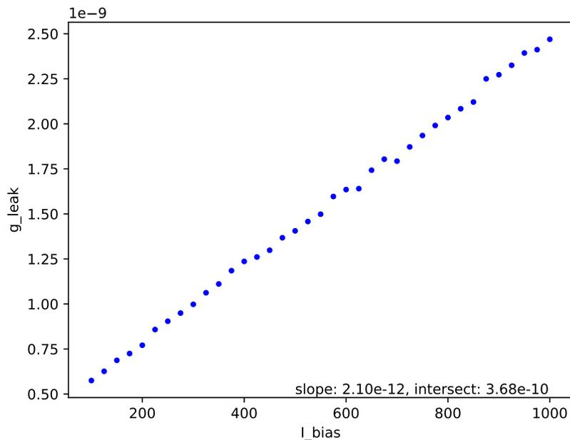
Figure 9: Measured  $g_{leak}$  over the whole DAC value range with parameters of the linear fit
