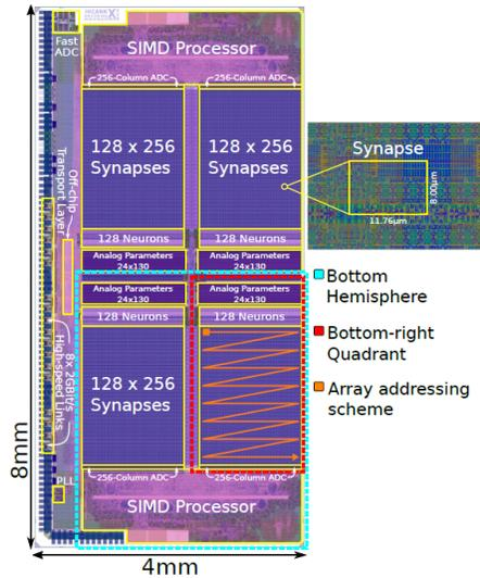
Figure 1: Schematic setup of the BrainScaleS-2 chip [3]
