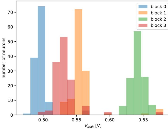
Figure 3: The histograms which contain the  $V_{leak}$  values of all 128 neurons of each block show significant deviations
