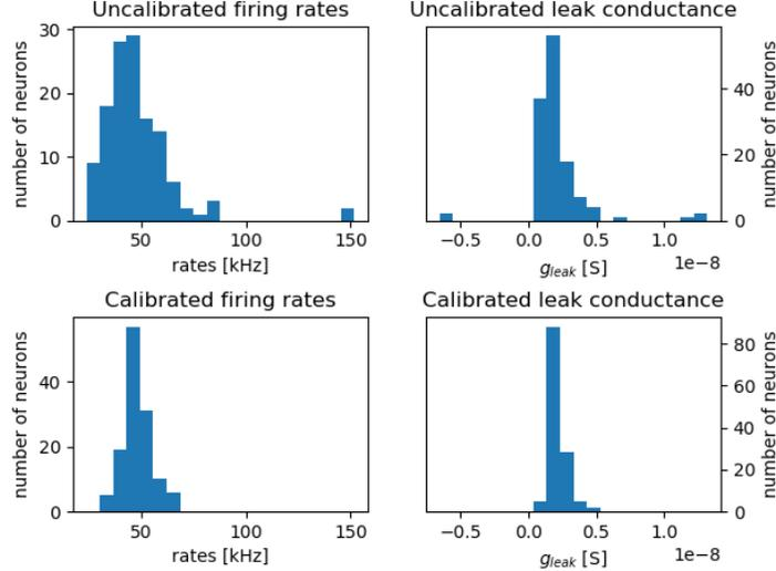
Figure 11: The uncalibrated setup (top) has a firing rate of  $47 \pm 18$  kHz and a leak conductance of  $(2.1 \pm 2.2) \times 10^{-9}$  S while the calibrated setup (bottom) has a value of  $48 \pm 7$  kHz for the firing rate and  $(2.1 \pm 0.7) \times 10^{-9}$  S for  $g_{leak}$ .
