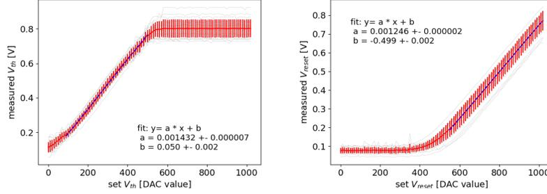
Figure 5:  $V_{th}$  (left) and  $V_{reset}$  (right) for 30 different neurons over the whole DAC value range, containing single runs (gray), mean (red) and linear fit (blue)
