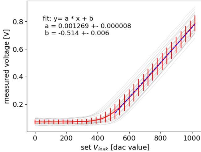
Figure 4: The gray lines show the  $V_{leak}$  values for 30 different neurons over the whole DAC value range, the red line is the mean of the single runs and used for the linear fit (blue)
