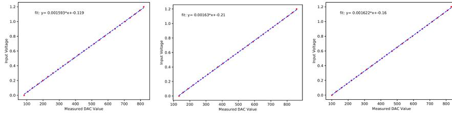
Figure 6: MADC characterization for setup 62 (left), setup 68 (middle) and setup 69 (right) with the respective linear translation fit (blue)
