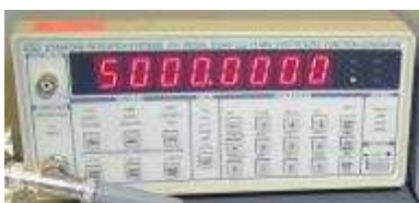
a) Frequenzgenerator SRS-DS340 von Stanford Research Systems
