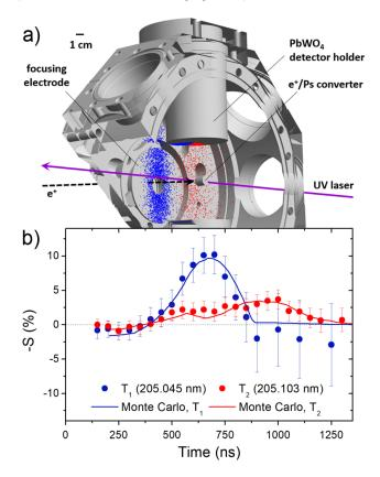
Figure 2: a) Distributions of Ps impact positions, shown superimposed to the 3D drawing of the chamber walls, for the  $T_1 = 175.6$  °C (blue circles) and  $T_2 = 172.4$  °C (red circles) setpoints, emphasizing the different
