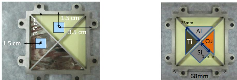
**Figure 7.** Left: setup used to measure the vertex resolution. Half of the surface is covered by a 20  $\mu\text{m}$  thin stainless steel foil. The blue squares indicate the scanning area used for the present analysis. Right: arrangement of foils to determine the annihilation multiplicities in various metals.
