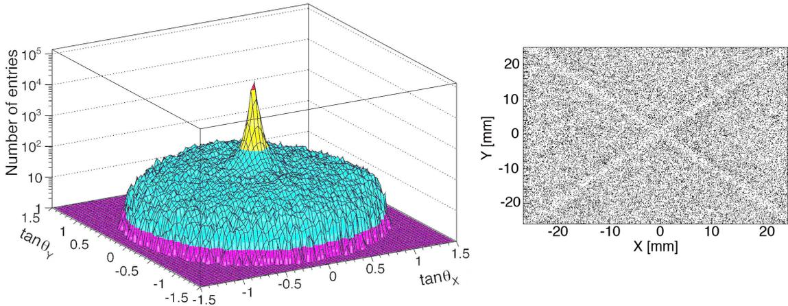
**Figure 5.** Left: angular distribution of annihilation tracks. Plotted are the tangents of the projected track angles. Right: spatial distribution of large angle tracks in an area of  $5 \times 5 \text{ cm}^2$  around the center.
