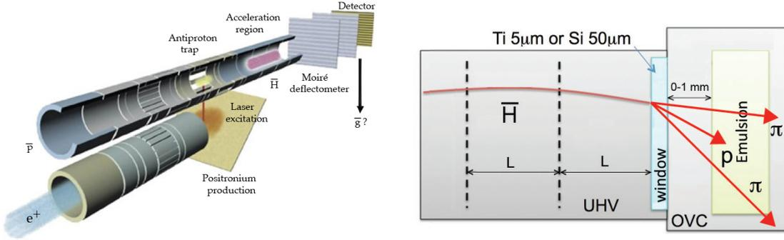
**Figure 1.** Left: sketch of the AEgIS apparatus. The  $\bar{\text{H}}$ -atoms are produced in the  $\bar{p}$ -trap in a 1 T field. Not shown are the  $\bar{p}$  and  $e^+$  capture traps in the 5 T magnet at the entrance of the apparatus. Right: Schematics of the AEgIS detectors. The vertex detector is made of a thin annihilation foil followed by nuclear emulsions. A time of flight detector (not shown) is needed to measure the velocity of the  $\bar{\text{H}}$  atoms.
