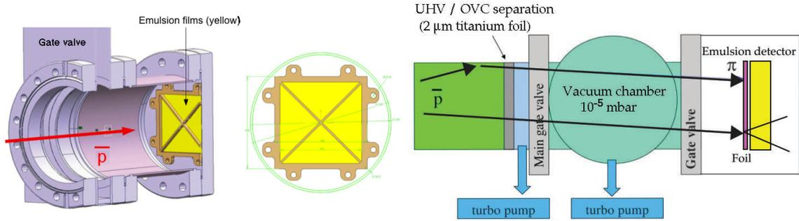
**Figure 3.** Left: vacuum chamber containing the emulsion detector. Right: beam line setup. Secondary particles (mainly pions) are generated by antiprotons annihilating in the upstream part of the AEGIS apparatus or directly in the emulsion detector.
