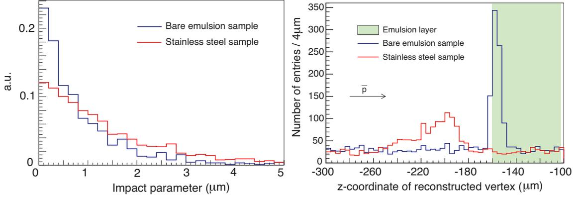
**Figure 8.** *Left: impact parameter distribution for annihilation on the bare emulsion surface (standard gel) and in the stainless steel foil. The histograms are normalized to the same area. A resolution of  $\sim 1 \mu\text{m}$  can be achieved for the  $\bar{g}$ -measurement. Right: vertex resolution in the  $z$ -direction (perpendicular to the surface).*
