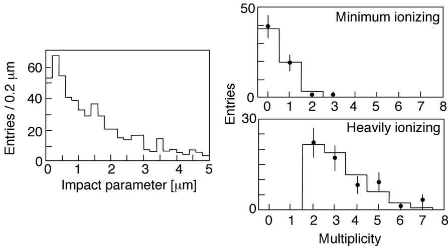
**Figure 10.** Measured impact parameter distribution for a  $6 \mu\text{m}$  aluminium foil (left) and multiplicity distribution for 60 events annihilating on the surface of the foil, for minimum ionizing and for heavily ionizing particles. The histogram is the Monte Carlo prediction from CHIPS.
