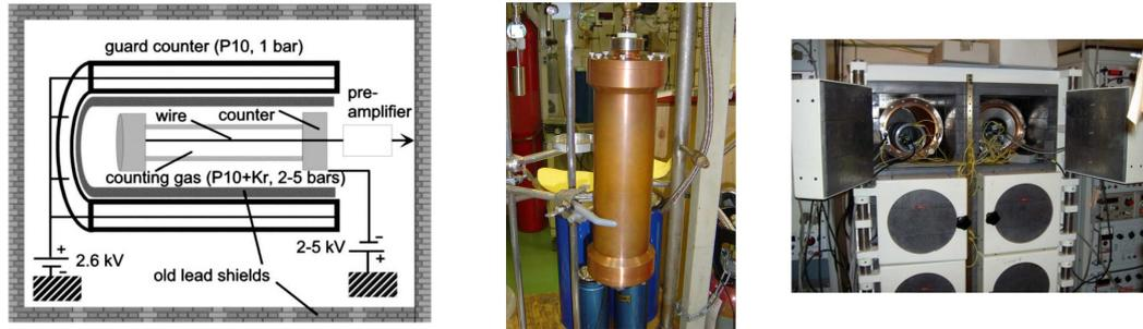
Figure 1.7.: Apparatus for measuring  $^{39}\text{Ar}$  by Low-Level-Decay-Counting in Bern [14].
