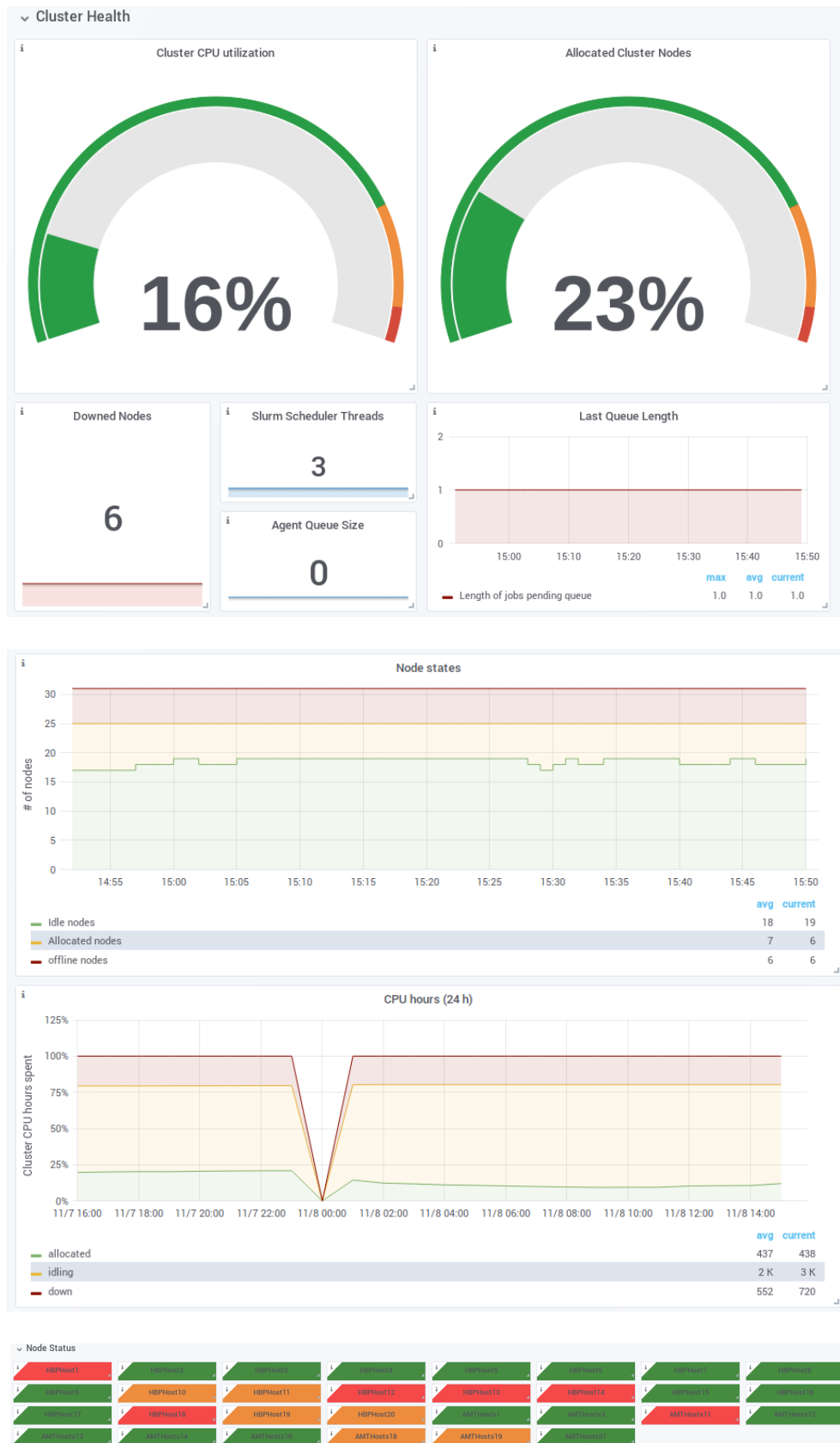
Figure 5: The first row is designed so that the health of the Slurm cluster can be assessed immediately.
