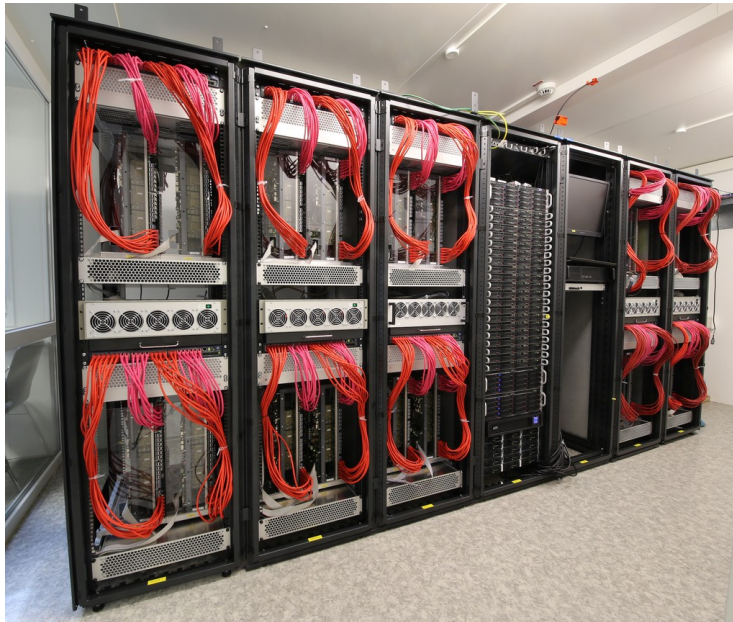
Figure 2: Photo of current NM-PM 1 setup. Wafer modules are located near the top and bottom of the lateral racks. Networking devices can be seen above each wafer module. Compute and storage nodes are situated in the center of the structure [2].
