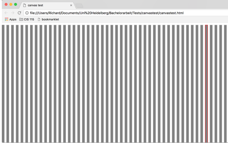
Figure 2: An example of a performance test using HTML canvas. A large number of simple stripes was drawn and pan&zoom as well as mouseover effects tested.
