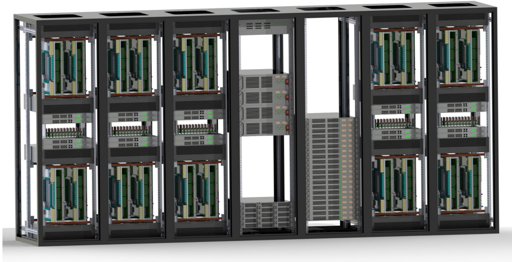
Figure 1.1.: Illustration of the HBP NM-PM1 system. The neuromorphic part is distributed over five racks containing four wafer modules each. A 20-node compute cluster including one storage server as well as two front-end nodes is located in the fourth rack (from the left); in the rendering, the compute nodes are located in the fifth cabinet. Communication between the individual wafer modules and compute nodes relies on multiple Gigabit Ethernet links that are aggregated to 10-Gigabit Ethernet. A backbone switch located on top of the compute cluster interconnects the compute nodes, the wafer switches and provides an uplink to the institute. Image by Dan Husmann.
