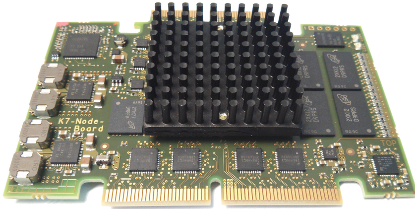
Figure 1.3.: FPGA communication PCB (FCP) used in the production-type HMF and NM-PM1 systems. The bottom connector is plugged into the Main-PCB. Host connectivity is provided by four wafer I/O PCBs (two horizontal and two vertical versions) that combine 12 FCPs each. Every FCP carries 1 GiB DRAM for spike data and 256 MB for communication buffers. For details see HBP SP9 Specification [2014].
