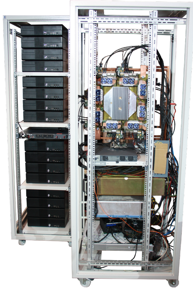
Figure 1.4.: Photograph of the first wafer prototype setup (right) together with the HMF compute cluster (left). All measurements using any part of the wafer module have been performed on this prototype. For a description of the differences between production-type and prototype wafer module see section 1.1.6. Details on the non-neuromorphic (or conventional) part, i.e. compute cluster and data network, can be found in sections 1.2 and 1.3.
