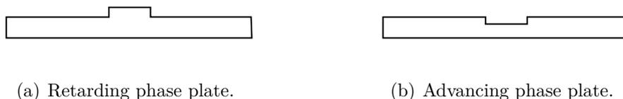
Figure 4.1: Schematical representation of the two possible phase plate design.
