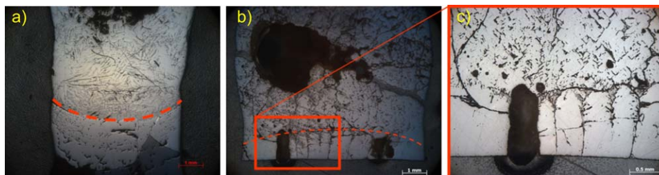
Fig. 4. Vertical section through the end of crystal (bottom) showing: (a) a concave crystal-melt interface for downward growth, (b) a convex interface for upward growth and (c) scale up of (b) showing cellular growth of the crystal-melt interface ahead the molten zone (top).
