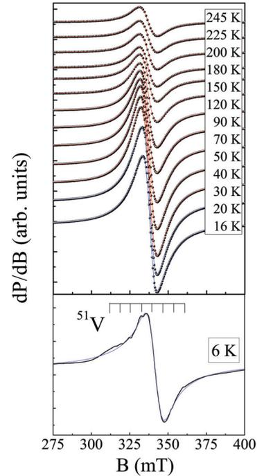
FIG. 3. (Color online) Temperature evolution of the first derivative X-band absorption for powder sample BaVSi<sub>2</sub>O<sub>7</sub> sample: points are experimental data; solid lines are the result of fitting by sum of two Lorentzians in accordance with Eq. (2). The spectra are shifted with respect to each other for clarity.
