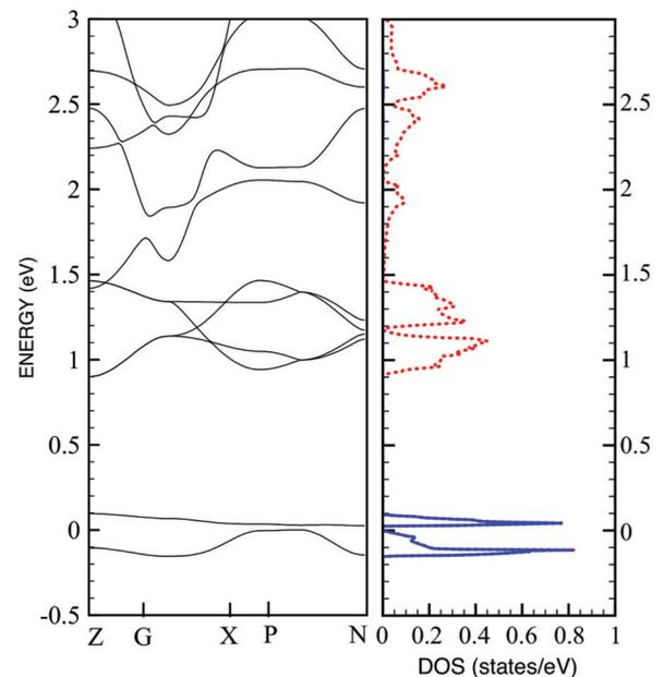
FIG. 9. (Color online) Band structure (left panel) and partial densities of states (right panel) obtained from LDA calculations. The solid and dashed lines are the density of states of  $3d$ - $xy$  and the total density of  $3d$  states, respectively. The Fermi energy corresponds to 0 eV.
