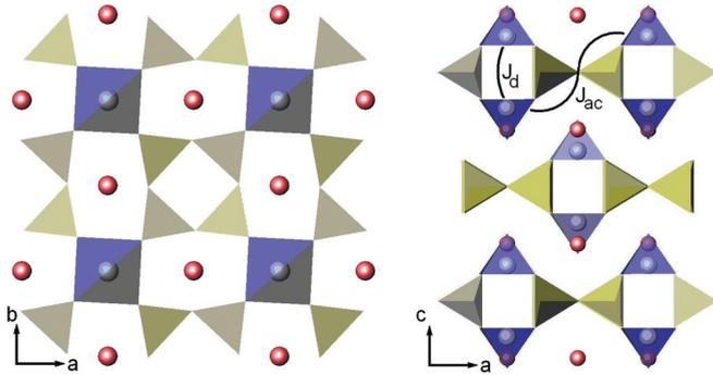
FIG. 1. (Color online) The crystal structure of  $\text{BaVSi}_2\text{O}_7$  (cf. Ref. 10). Left panel: the intralayer topology; right panel: the interlayer arrangement. The apparent square and triangular polyhedra represent  $\text{VO}_5$  pyramids and  $\text{SiO}_4$  tetrahedra, respectively.  $\text{Ba}^{2+}$  ions (circles) occupy the interlayer. The arcs  $J_d$  and  $J_{ac}$  denote intradimer and interdimer exchange pathways, respectively.
