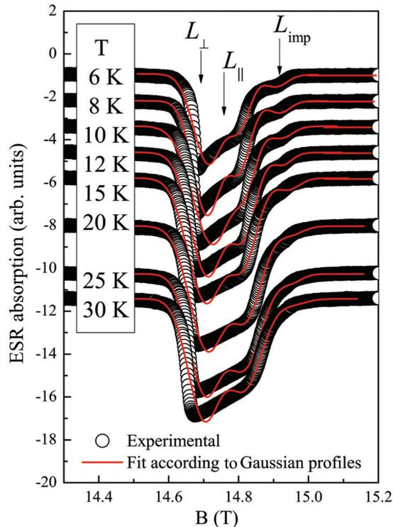
FIG. 4. (Color online) Evolution of the ESR spectra with temperature at 405 GHz for powder sample  $\text{BaVSi}_2\text{O}_7$ : the circles are experimental data; lines are the results of fitting according to Gaussian lineshape profile [Eq. (3)]. The spectra are shifted with respect to each other for clarity.
