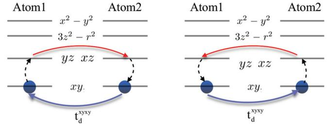
FIG. 10. (Color online) Examples of virtual hopping processes that contribute to the intradimer symmetric anisotropic exchange interactions  $\Gamma_d^{xx}$  and  $\Gamma_d^{yy}$ . Spheres denote the  $3d$  electrons that can hop between sites (lower solid lines). The hoppings between empty orbitals are visualized by the upper solid lines. The dashed lines correspond to the mixing of the occupied and empty orbitals due to the spin-orbit coupling.
