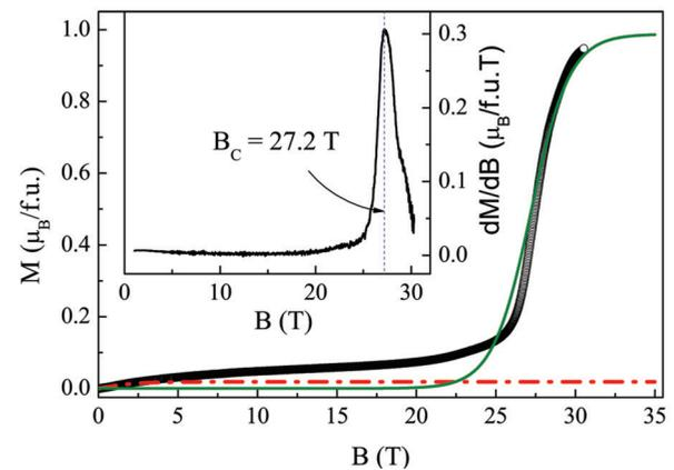
FIG. 7. (Color online) The magnetization curve of BaVSi<sub>2</sub>O<sub>7</sub> at 1.6 K. The defect/impurity contribution approximated by the Brillouin function is shown by the dash-dotted line. The solid line represents the fit of the  $M(B)$  curve in a noninteracting dimer model. The inset represents the derivative of the magnetization curve; the critical magnetic field  $B_C = 27.2$  T is indicated by the vertical dashed line.
