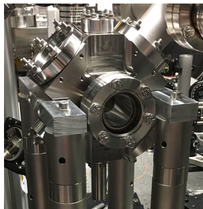
(a) Side view of the 2D MOT chamber.
