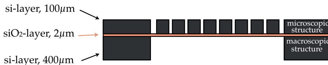
Figure 4.6: Sketch of a cross-section through a SOI-wafer. For our purposes, we use a 2\ \mu\text{m} -thick insulator layer of silicon-oxygen, \text{SiO}_2 . The ‘microscopic structure’ is etched into the 100\ \mu\text{m} -thick upper silicon-layer, and the ‘macroscopic structure’ is etched into the 400\ \mu\text{m} -thick bottom layer. This picture has been received from [75].
