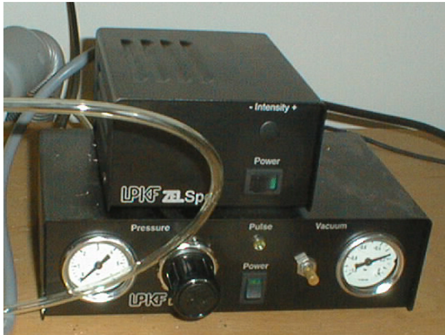
Figure 3.6: Station for pressure, vacuum and light
