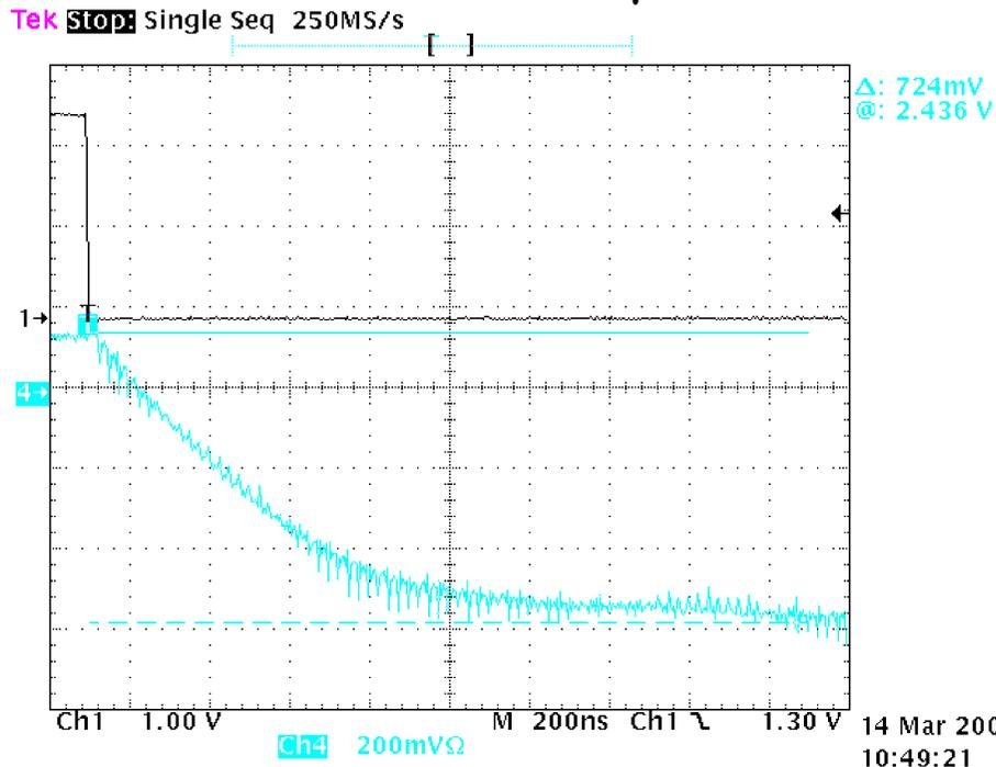
Voltage controlling delay settles  $2\mu\text{s}$  after reset of the circuit
