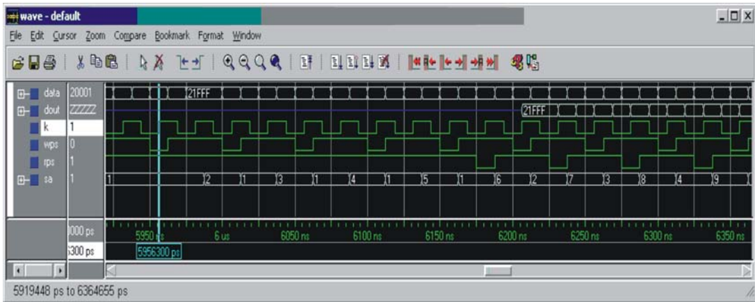
Figure 6-14 Simulation of data to (labelled data) and from (labelled dout) the QDR chip.
