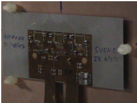
Figure 6.51: Target hybrid with 3 Beetle chips for SEU irradiation test.
