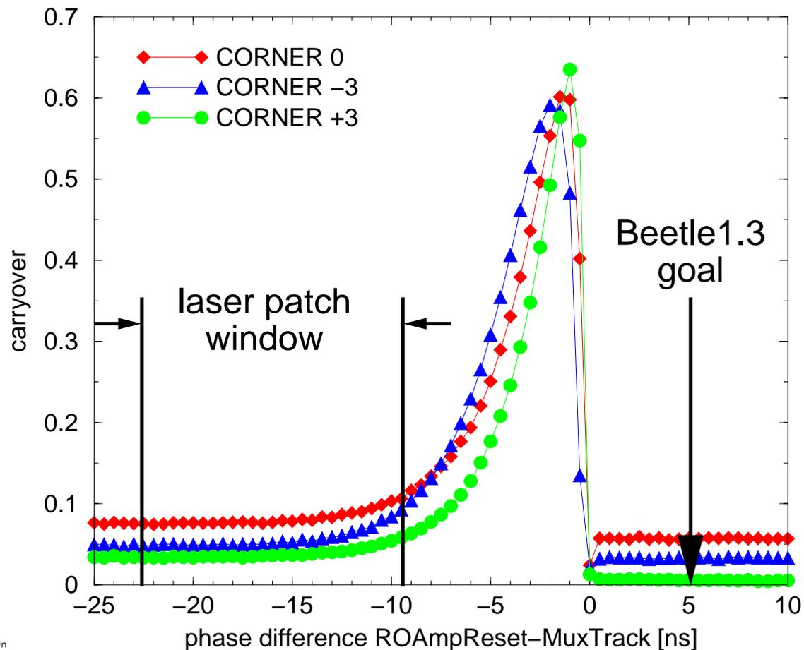
**Modification in Beetle1.3: analog delay of MuxTrack by 5 ns** ↑
