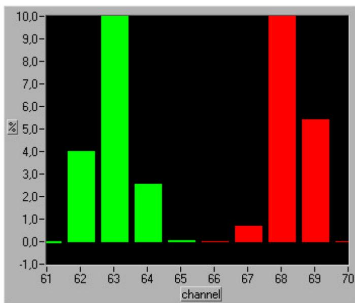
Testpulse (63. & 68) is standardised to 100%
