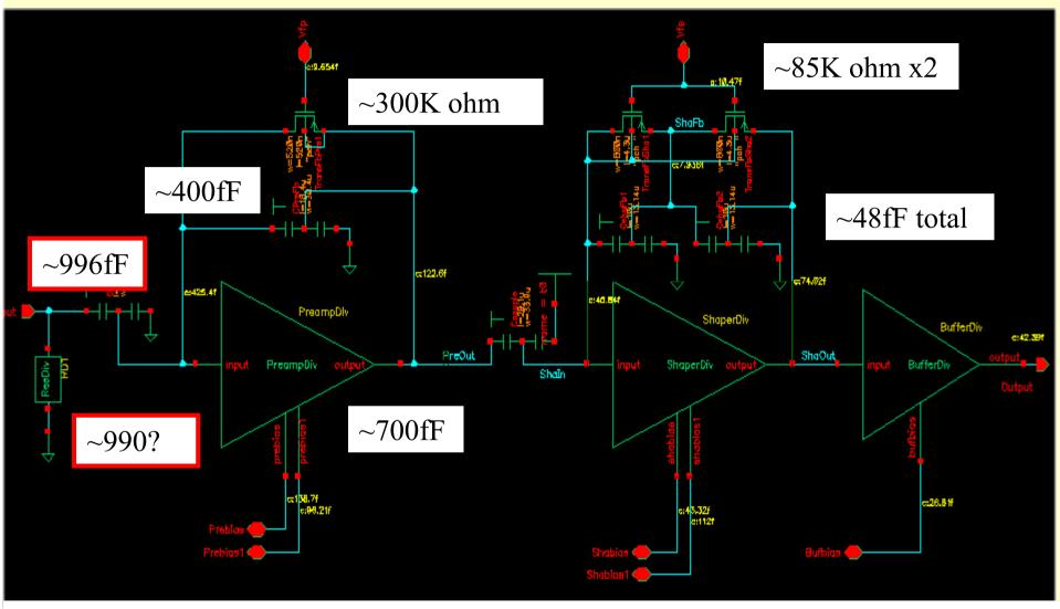
Red box means different to the standard Beetle1.2
