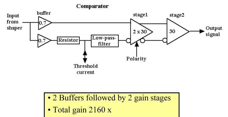
• Output polarity switch
