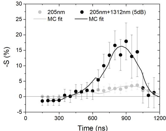
Figure 4: The experimental curve of the  $-S$  parameter ( $= (A^{\text{UV+IR}}(t) - A^{\text{off}}(t))/A^{\text{off}}(t)$ ) measured in the empirically-determined optimal 1312.2 nm laser intensity, compared to the reference  $-S$  obtained without the IR laser.
