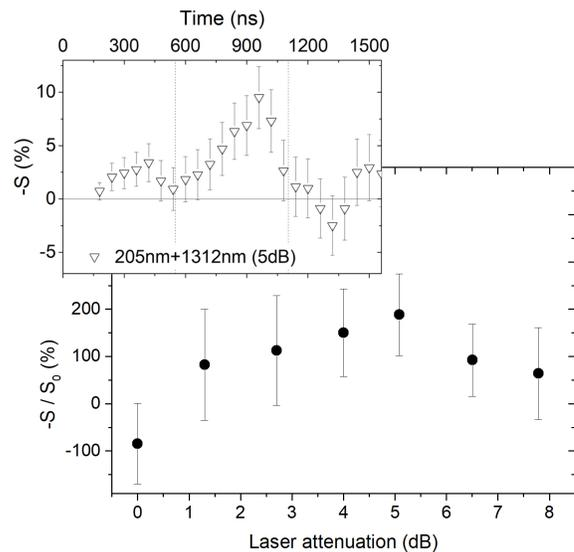
Figure 3: The ratio  $-\bar{S}/\bar{S}_0$  between the total  $S$  parameters, as defined in the text, versus the attenuation in dB of the IR laser pulse starting from the maximum energy  $405 \mu\text{J}$  (black points): Top inset: the  $-S(t)$  parameter in the case of the 5 dB attenuation point.
