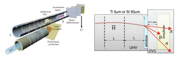
**Figure 1.** Left: sketch of the AEgIS apparatus. The  $\overline{H}$ -atoms are produced in the  $\overline{p}$ -trap in a 1 T field. Not shown are the  $\overline{p}$  and  $e^+$  capture traps in the 5 T magnet at the entrance of the apparatus. Right: Schematics of the AEgIS detectors. The vertex detector is made of a thin annihilation foil followed by nuclear emulsions. A time of flight detector (not shown) is needed to measure the velocity of the  $\overline{H}$  atoms.
