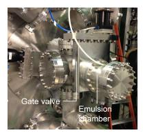
**Figure 4.** Photograph of the emulsion chamber at the downstram end of the AEgIS apparatus.
