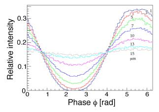
**Figure 15.** Simulated intensity distribution of reconstructed vertices for various vertex resolutions between 1 and 15  $\mu$ m.
