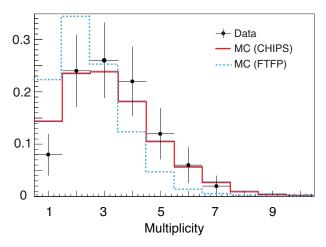
**Figure 11.** Multiplicity distribution of ejectiles emitted isotropically into a solid angle  $2\pi$  in antiproton annihilation at rest in emulsions (new gel), for data and for Monte Carlo predictions based on CHIPS (red continuous histogram) and FTFP (blue dashed histogram). The distributions are normalized to one.
