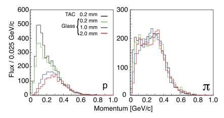
**Figure 13.** Momentum distribution of basetracks for protons (left), respectively pions (right), for various glass thicknesses and for a plastic (TAC) base.
