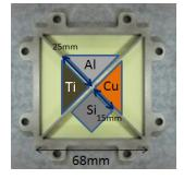
**Figure 7.** Left: setup used to measure the vertex resolution. Half of the surface is covered by a 20  $\mu$ m thin stainless steel foil. The blue squares indicate the scanning area used for the present analysis. Right: arrangement of foils to determine the annihilation multiplicities in various metals.
