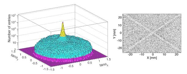
**Figure 5.** Left: angular distribution of annihilation tracks. Plotted are the tangents of the projected track angles. Right: spatial distribution of large angle tracks in an area of  $5 \times 5$  cm<sup>2</sup> around the center.
