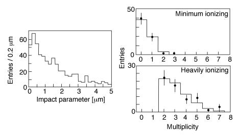
**Figure 10.** Measured impact parameter distribution for a 6 µm aluminium foil (left) and multiplicity distribution for 60 events annihilating on the surface of the foil, for minimum ionizing and for heavily ionizing particles. The histogram is the Monte Carlo prediction from CHIPS.
