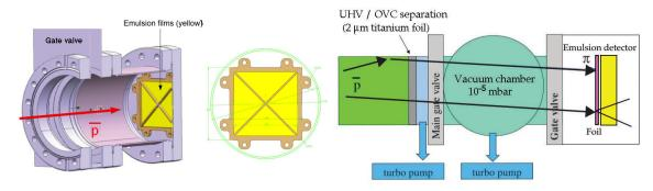
**Figure 3.** Left: vacuum chamber containing the emulsion detector. Right: beam line setup. Secondary particles (mainly pions) are generated by antiprotons annihilating in the upstream part of the AEgIS apparatus or directly in the emulsion detector.
