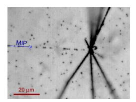
**Figure 6.** Typical tracks from minimum ionizing particles and from fragments emerging from the annihilation vertex, observed in the standard gel (left) and in the new gel (right).
