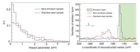
**Figure 8.** Left: impact parameter distribution for annihilation on the bare emulsion surface (standard gel) and in the stainless steel foil. The histograms are normalized to the same area. A resolution of  $\sim 1~\mu m$  can be achieved for the  $\bar{g}$ -measurement. Right: vertex resolution in the z-direction (perpendicular to the surface).
