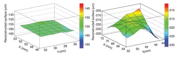
**Figure 9.** Topography of the emulsion surface (left) and of the stainless steel foil (right). The vertical scale refers to the distance in  $\mu$ m from the vertex to the center of the base.
