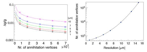
**Figure 16.** Left: relative precision on g vs. number of annihilation vertices for various vertex resolutions from 1 to 10  $\mu$ m. Right: Number of annihilation vertices required to reach 1% on  $\Delta g/g$ , vs. vertex resolution (the curve is an eyeball fit to the points).
