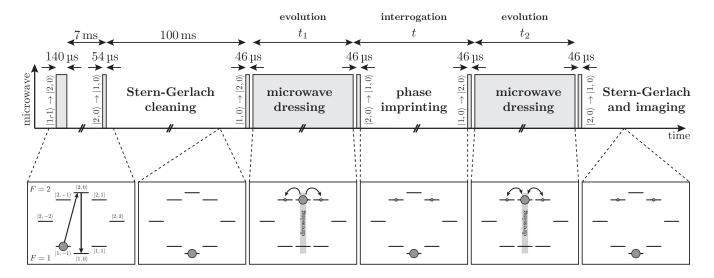
Figure S1. Timing diagram. Microwave pulses used for state preparation and energy level shifting (dressing) are indicated in the upper panel. The lower panels show the energy levels at each stage with the linear Zeeman shift subtracted.
