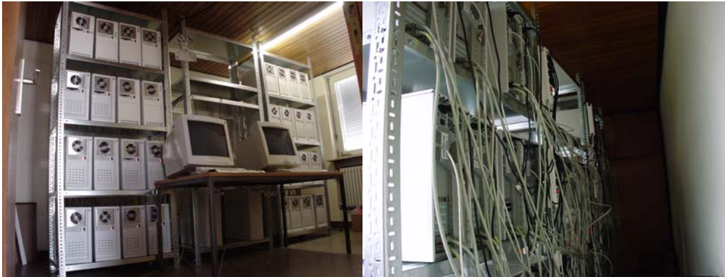
Figure 7.1: 30 nodes out of 32 Linux computers are connected to a 10 \times 3 torus. The picture on the right shows the SCI cabling.
