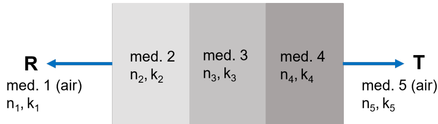
Figure 3.4. Schematic of the Transfer Matrix Method (TMM) for optical generation calculation in Sentaurus Device.
