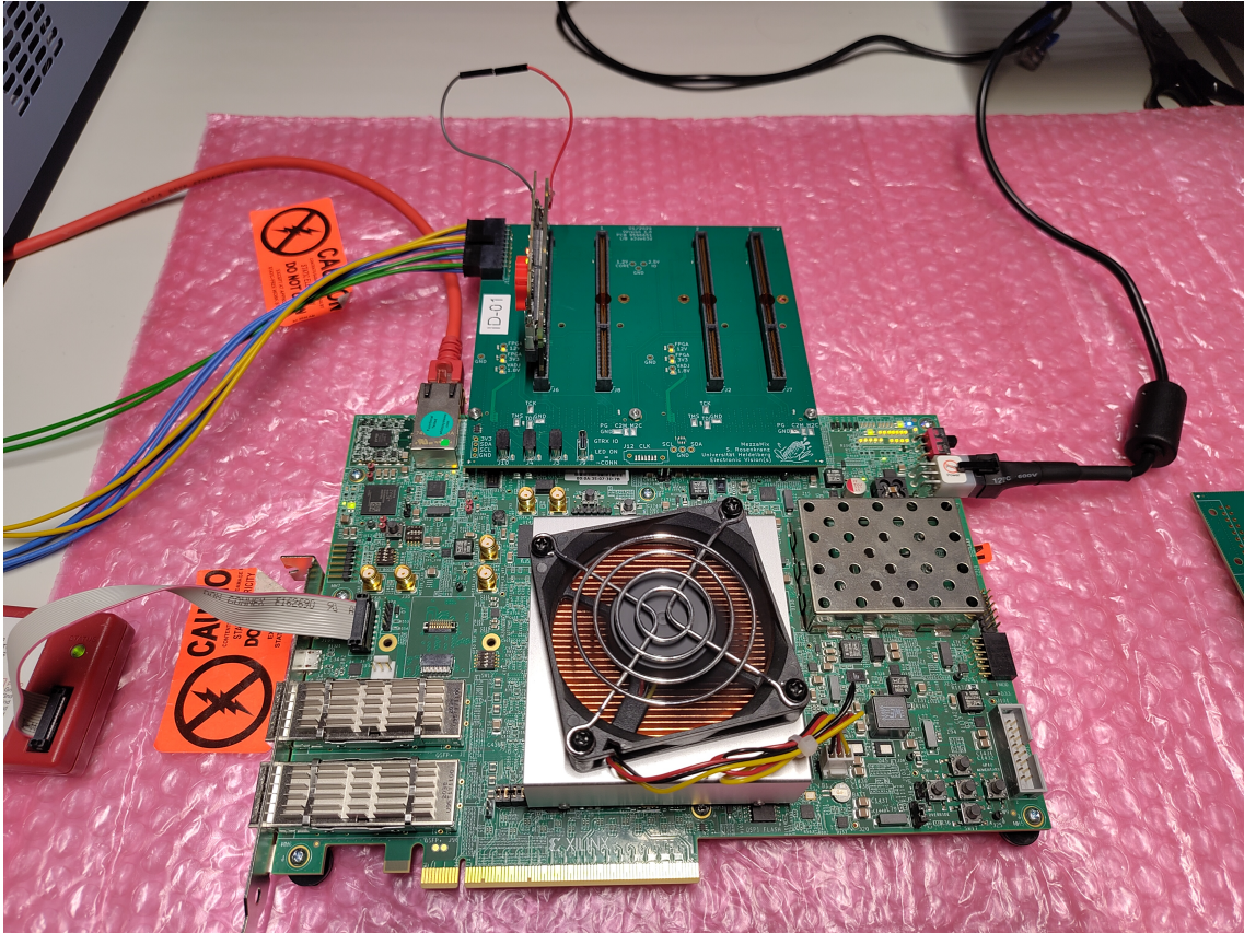
Figure 2.9: Top-view photograph of the assembled multi-chip setup during operation with a single HICANN-X.
