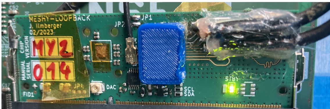
Figure 2.3: The “meshy-loopback” chip carrier. The chip and its I/O cells are placed under the blue cover. On the right, the two lemo cables are soldered to the PHY connections and fixed with hot melt adhesive. Left of the blue cover, the V_{\text{Ref}} pad is connected to the multimeter via a mini-coax connection. Not seen on the reverse side is the soldered active differential probe.
