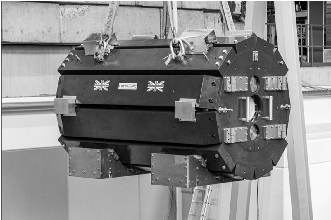
Figure 3.10: Mu3e solenoid magnet delivery at PSI. The whole magnet is shielded by a 27-ton iron coat to reduce the stray field to < 5 mT at a distance of 1 m. Figure from [83].
