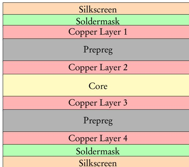
Figure 5: Typical four layer stackup PCB
