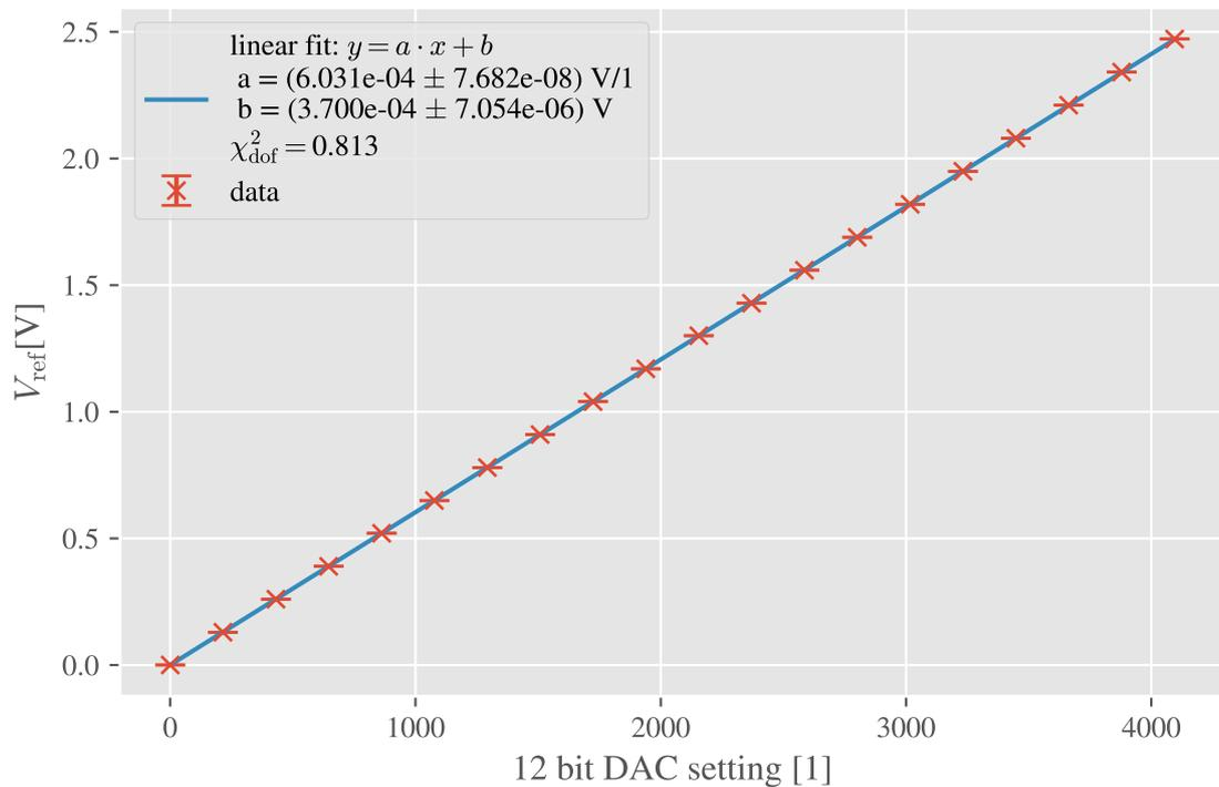
Figure 19: DAC calibration sweep at  $T_{\text{amb}} = 25 \text{ }^\circ\text{C}$
