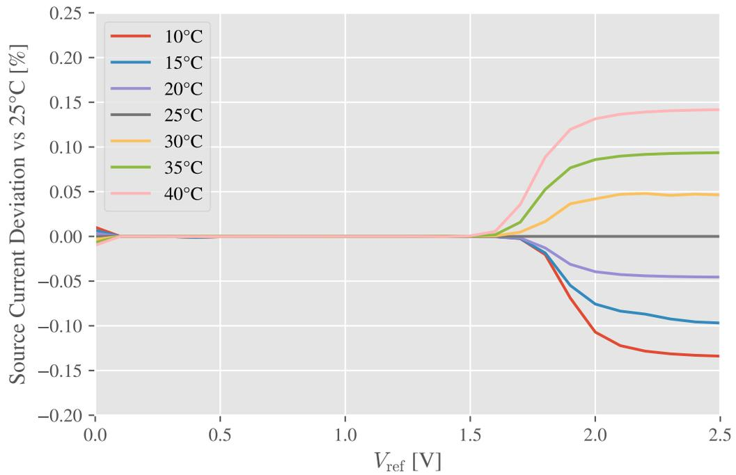
Figure 17: Temperature dependent deviation of source current as a function of  $V_{ref}$  at  $V_{op} = 0.5$  V — normalized to 25 °C
