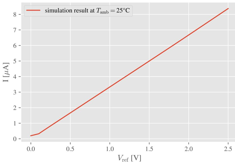
Figure 16: Simulation results for reference voltage sweep with  $V_{\text{op}} = 0.53 \text{ V}$  at ambient temperature of  $25^\circ\text{C}$
