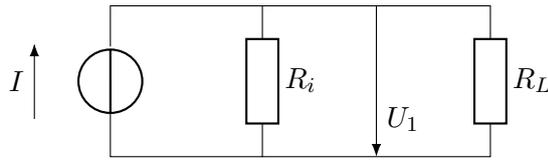
Figure 2: Idealized current source schematic
