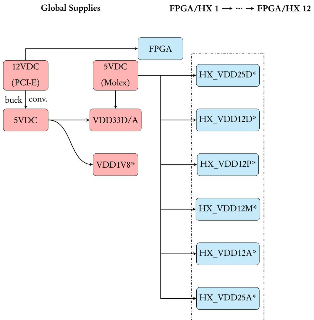
Figure 9: Power supply layout (\* current/voltage monitored)
