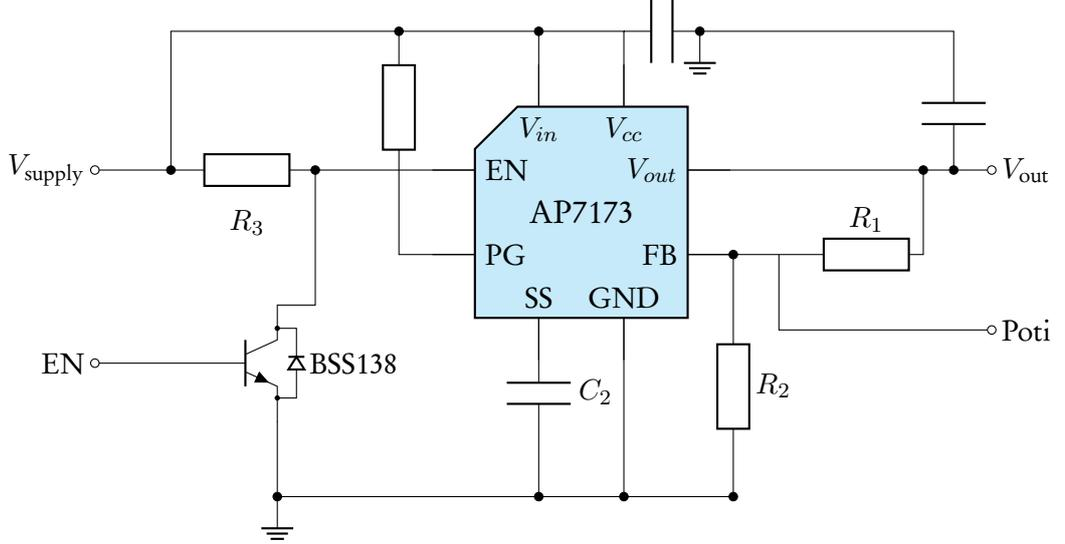
Figure 10: Simplified schematic of a HICANN LDO supply
