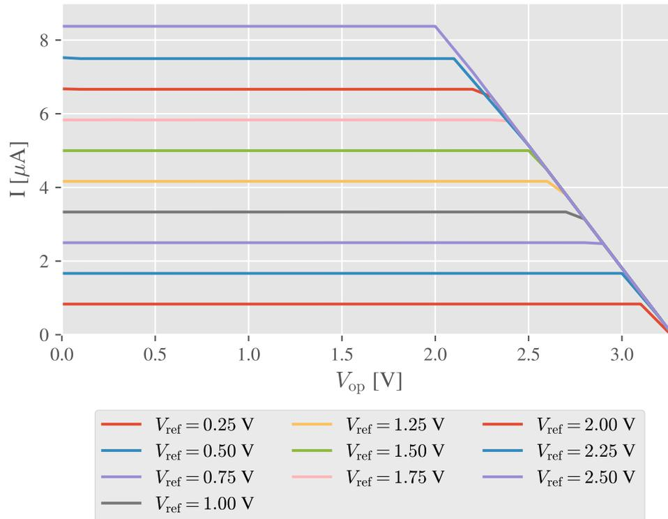
Figure 18:  $V_{op}$  sweep at  $T_{amb} = 25^\circ\text{C}$
