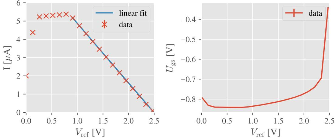
Figure 20: Reference voltage sweep at  $V_{\text{op}} = 0.53 \text{ V}$  and  $T_{\text{amb}} = 25 \text{ }^\circ\text{C}$
