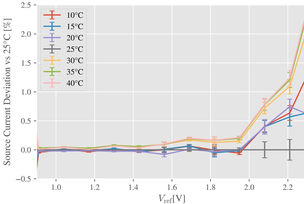
Figure 22: Temperature dependent deviation of source current as a function of  $V_{ref}$  at  $V_{op} = 0.53$  V, normalized to 25 °C
