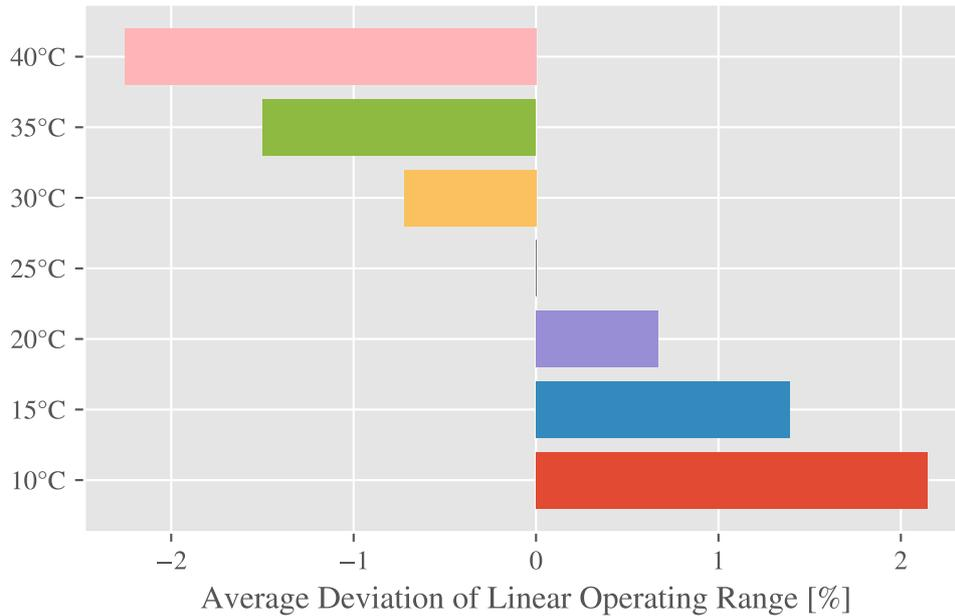
Figure 24: Average deviation of linear operating range due to ambient air temperature variation. Values indicate the change of the operating point where the source current collapses.
