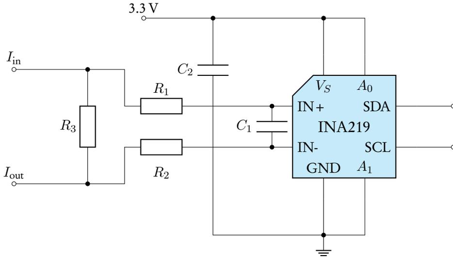
Figure 11: Current Measurement Schematic
