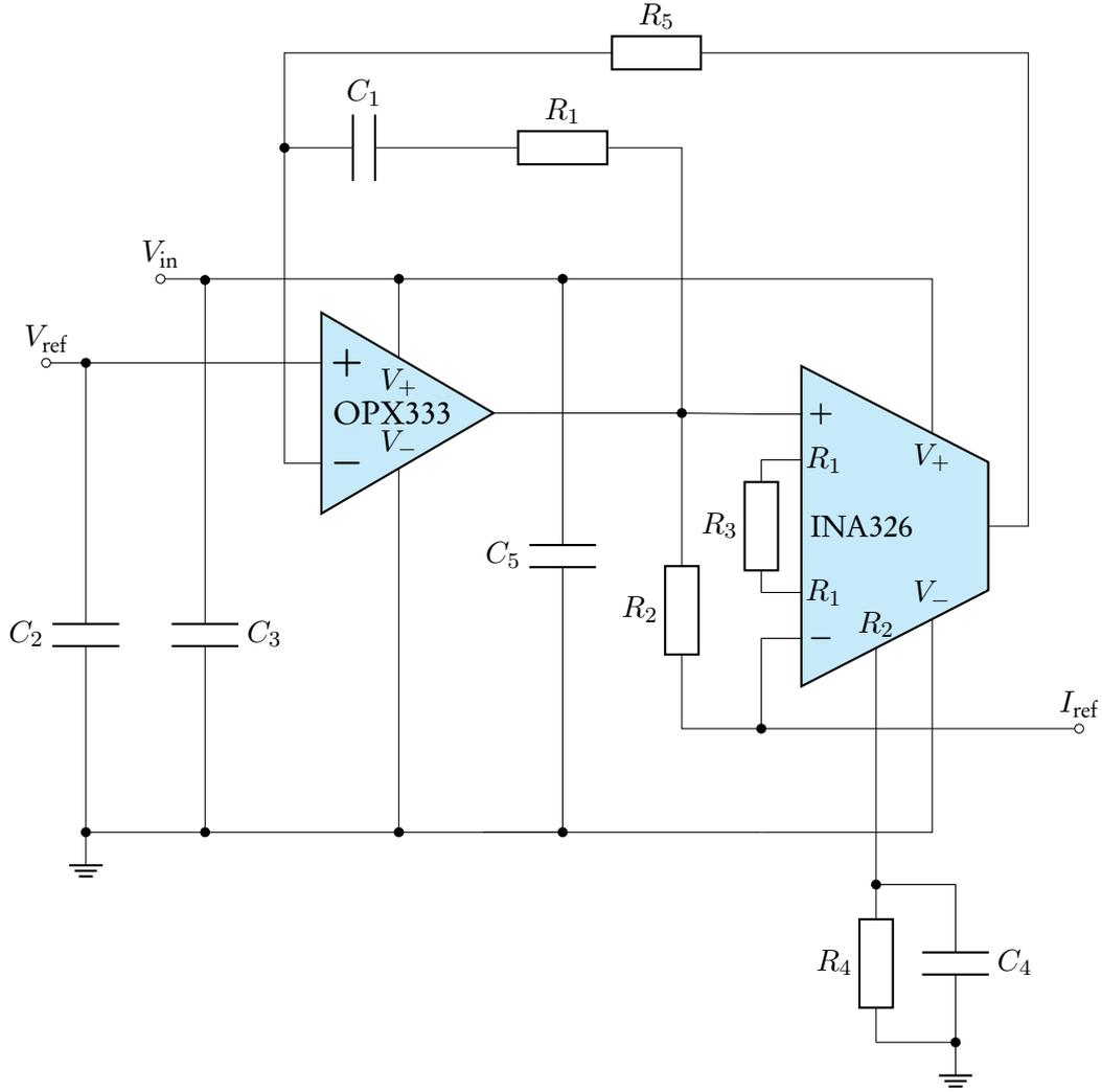
Figure 12: Reference Current Source Option A Schematic
