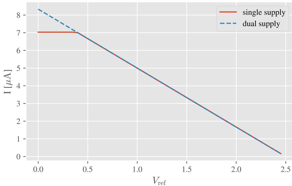
Figure 21: Simulation of single ( $V_- = 0\text{ V}$ ,  $V_+ = 2.5\text{ V}$ ) and dual supply ( $V_- = -2.5\text{ V}$ ,  $V_+ = 2.5\text{ V}$ ) configuration of the operational amplifier at  $V_{\text{op}} = 0\text{ V}$
