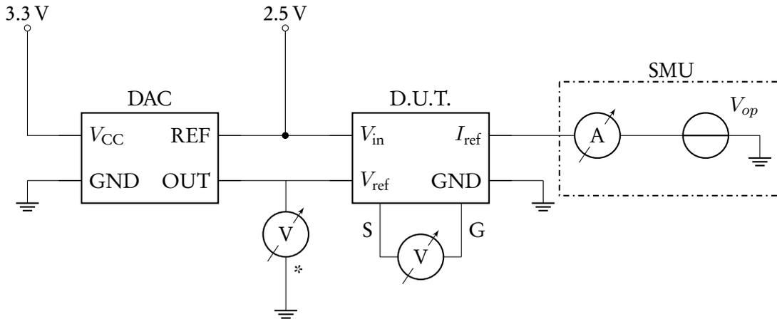
Figure 15: SMU measuring setup with current source as D.U.T.
