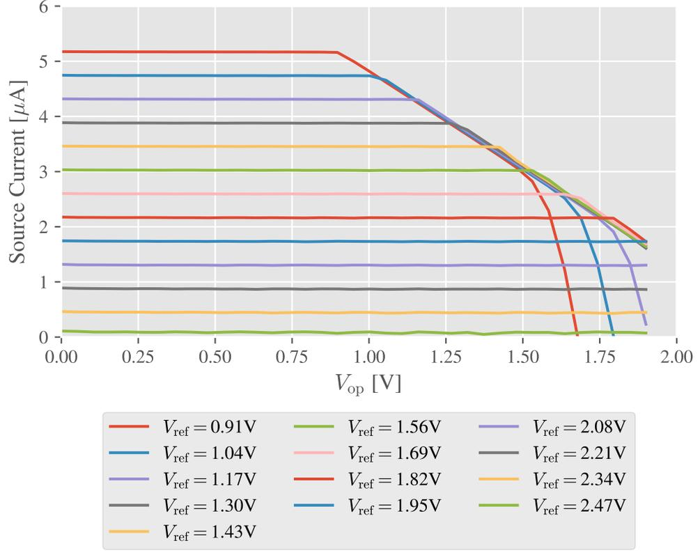
Figure 23:  $V_{op}$  sweep at  $T_{amb} = 25^\circ C$
