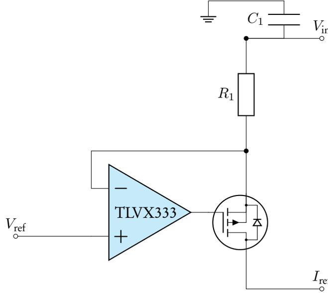
Figure 13: Reference Current Source Option B Schematic
