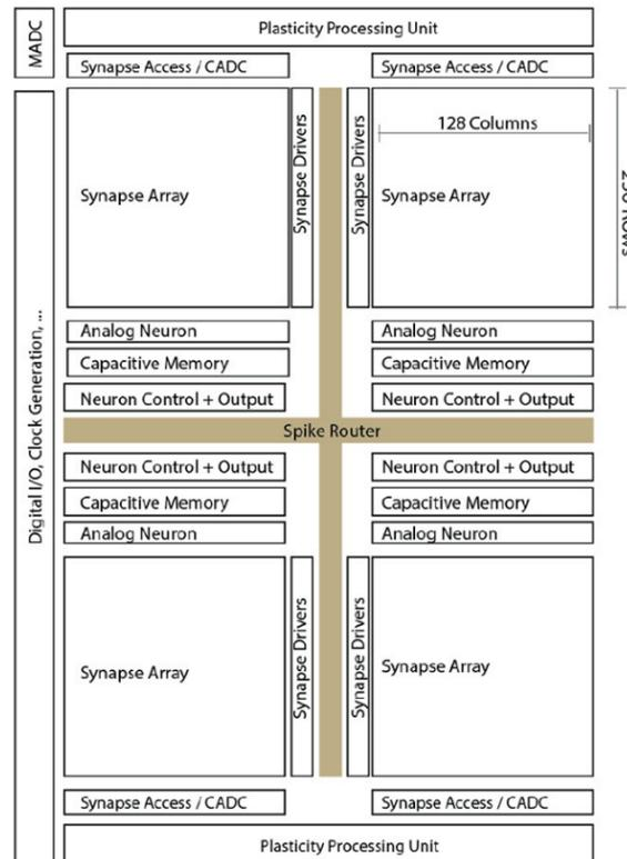
Figure 1: Schematic layout of the HICANN ASIC (Pehle et al. 2022)
