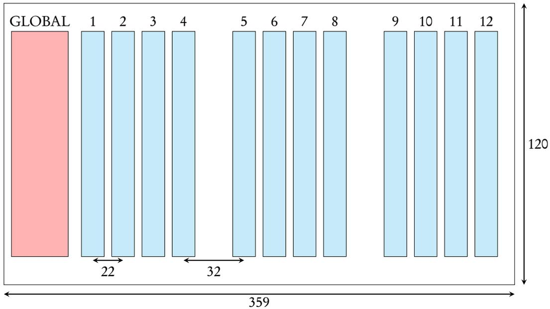
Figure 7: PCB schematic footprint (dimensions in millimeters)
