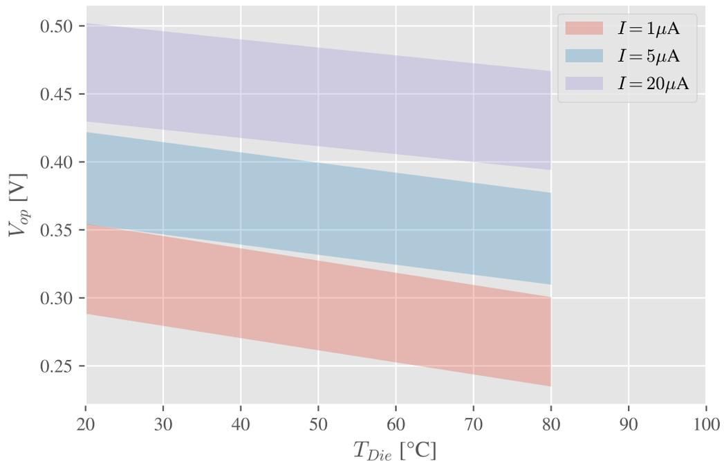
Figure 3: Simulation results of the voltage settling at the external reference input pin of the HICANN chip over all relevant corner variations (Ilmberger 2022)
