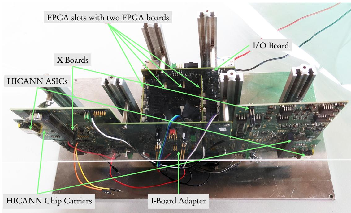
Figure 4: BSS-2 Cube setup with two fitted FPGAs
