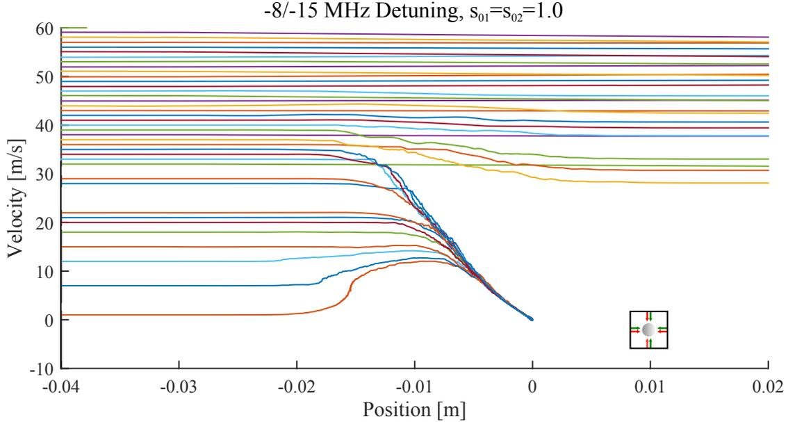
Figure 3.8: Numerical solution of the atom trajectories of  $^{38}\text{Ar}$  inside a double frequency MOT with time-dependent scattering rate (eq. 3.31).  $\delta_1 = -8$  MHz,  $\delta_2 = -15$  MHz,  $s_{01} = s_{02} = 1$ ,  $\frac{dB}{dz} \approx 10$  G/cm. Capture velocity  $v_c = 35$  m/s.
