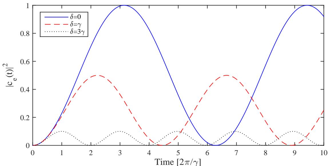
Figure 3.1: Rabi oscillations of the excited state  $|e\rangle$  for detunings  $\delta = 0$  (solid, blue),  $\gamma$  (dashed, red),  $3\gamma$  (dotted, black).
