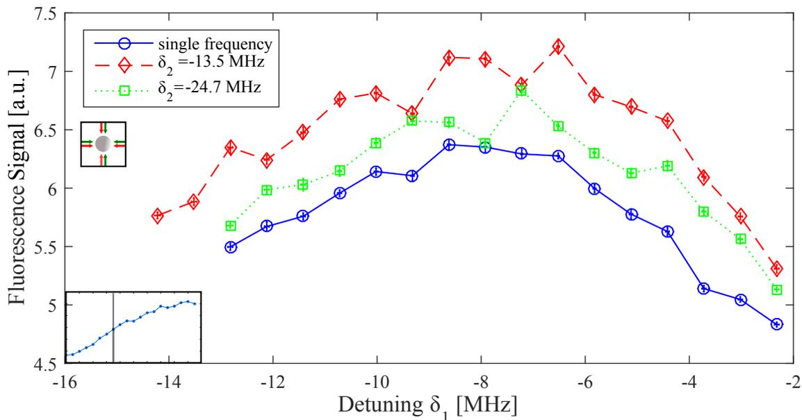
Figure 5.11: MOT fluorescence signal over detuning of the first frequency  $\delta_1$  for three different setups with  $s_{01} = 1.0$ . The solid (blue) curve displays the previously shown single frequency data as reference. Shown by the dashed (red) curve is the signal for  $\delta_2 = -13.5$  MHz and by the dotted (green) curve for  $\delta_2 = -24.7$  MHz. It is  $s_{02} = 0.4$  for both. All data was taken after 7 ms loading time.
