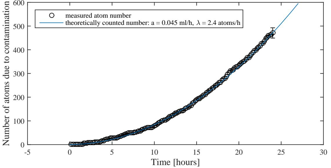
Figure 4.7: In recycling configuration measured contamination of a dead argon sample over time. Number of measured atoms shown by (black) circles, the solid (blue) curve displays the theoretically counted atom number for a count rate of  $\lambda = 2.4$  atoms/h and a contamination acceleration of  $a = 0.045$  ml STP/h. The error of the total atom number in the end is given by its squareroot (Poisson).
