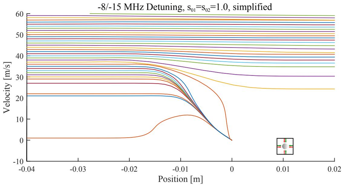
Figure 3.9: Numerical solution of the atom trajectories of  $^{38}\text{Ar}$  inside a double frequency MOT with time-independent scattering rate (eq. 3.34).  $\delta_1 = -8$  MHz,  $\delta_2 = -15$  MHz,  $s_{01} = s_{02} = 1$ ,  $\frac{dB}{dz} \approx 10$  G/cm. Capture velocity  $v_c = 36$  m/s.
