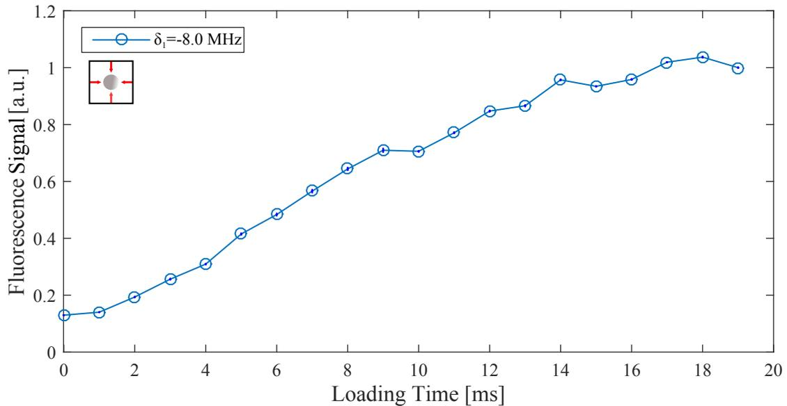
Figure 5.5: Loading curve: Fluorescence signal over loading time for the single-frequency MOT with  $\delta_1 = -8.0$  MHz,  $s_{01} = 1.0$ . Small icons displayed in the graph should indicate whether the single or double frequency MOT is shown.
