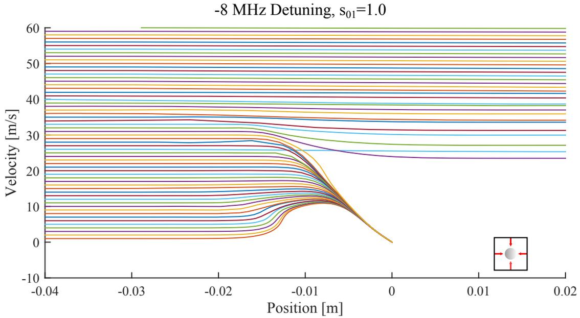
Figure 3.7: Numerical solution of the atom trajectories of  $^{38}\text{Ar}$  inside a single frequency MOT.  $\delta_1 = -8$  MHz,  $s_{01} = 1$ ,  $\frac{dB}{dz} \approx 10$  G/cm. Capture velocity  $v_c = 30$  m/s. Small icons displayed in the graph should indicate whether the single or double frequency MOT is shown.
