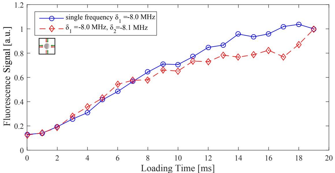
Figure 5.9: Loading curves for the single frequency case (solid, blue) and a double frequency configuration (dashed, red) whereas  $\delta_1 = -8.0$  MHz and  $\delta_2 = -8.1$  MHz,  $s_{02} = 0.6$ ,  $s_{01} = 1.0$ .
