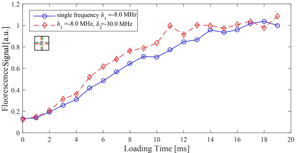
Figure 5.10: Loading curve with a high second frequency detuning of  $\delta_2 = -30.0$  MHz (dashed, red),  $s_{02} = 0.6$ ,  $s_{01} = 1.0$ . As a reference the single frequency data is shown by the solid curve (blue).
