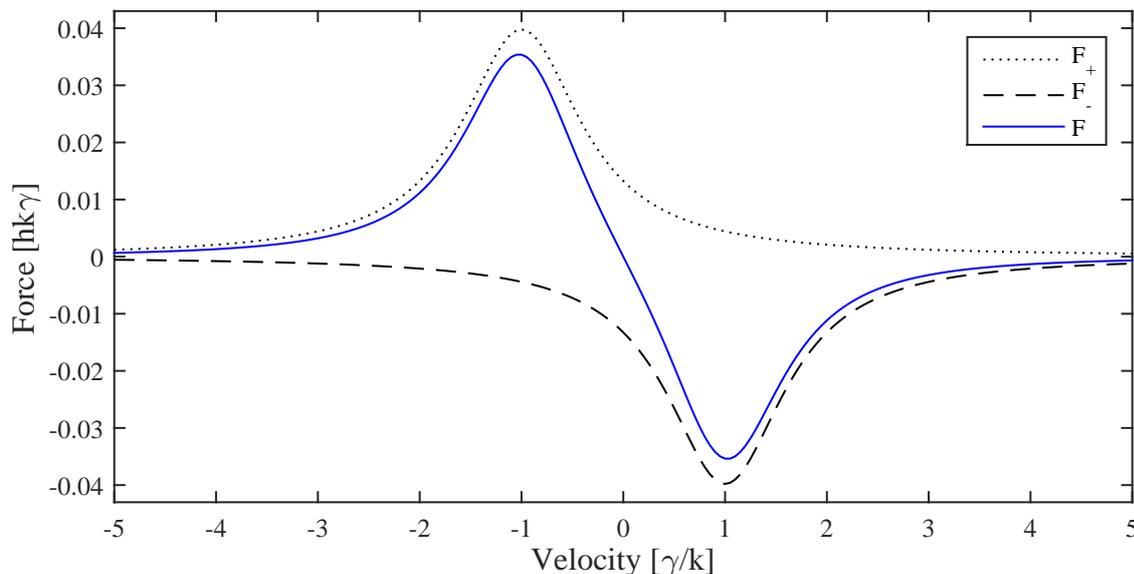
Figure 3.3: Forces on the atom in the one dimensional optical molasses depending on its velocity. Shown are the forces for the two counterpropagating laser beams  $F_+$  (dotted) and  $F_-$  (dashed) for  $\delta = \gamma$  and  $s_0 = 1$ . The solid (blue) line displays the sum of the two.
