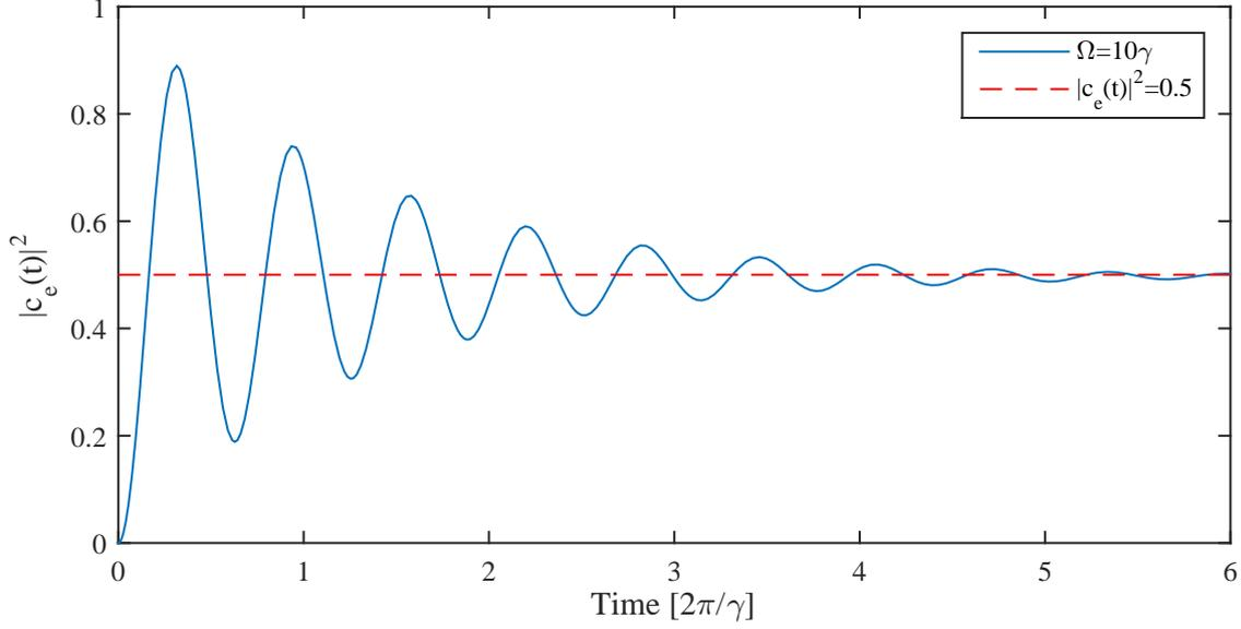
Figure 3.2: The solid (blue) curve shows the solution of a numerical calculation of  $\rho_{ee}$  with spontaneous emission included (from eq. 3.16). Here  $\delta = 0$  and  $\Omega = 10\gamma$  were chosen. The dotted (red) line displays the stationary solution  $\rho_{ee} = 0.5$  which is reached after the oscillations of the solid curve are fully damped.
