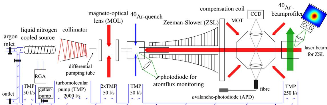
Figure 4.1: Scheme of the ATTA apparatus in Heidelberg. The flux of the atoms is directed from the source on the left side towards the MOT chamber on the right side. The figure includes the atom optical tools as well as the vacuum setup. Adapted from [4].
