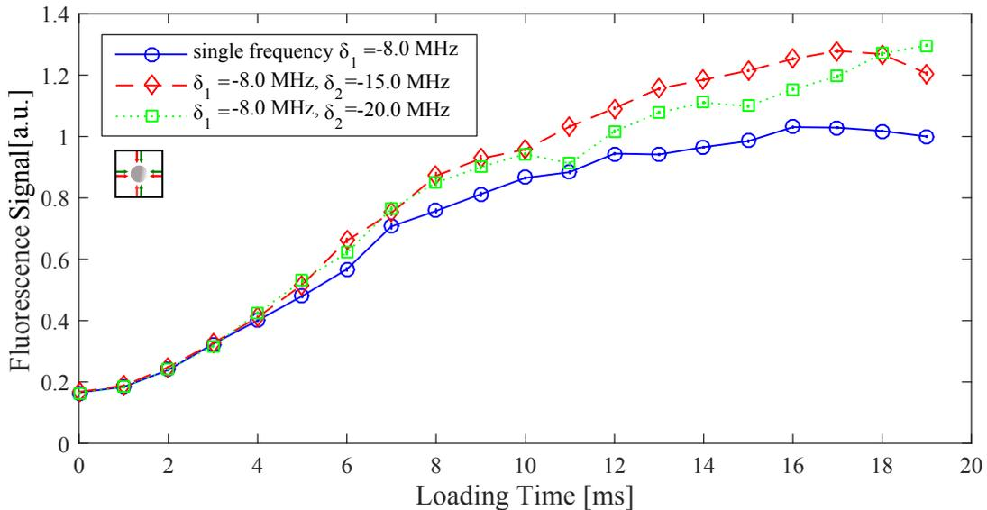
Figure 5.8: Loading curves for different detunings. Shown by the solid (blue) curve is the loading behaviour for the single frequency case from fig. 5.5 with  $\delta_1 = -8.0$  MHz and  $s_{01} = 1.0$ . The second frequency is introduced with a detuning of  $\delta_2 = -15.0$  MHz, shown by the dashed (red) curve, and  $\delta_2 = -20.0$  MHz, shown by the dotted (green) curve. For both  $\delta_2$  the power was set to  $s_{02} = 0.6$ .
