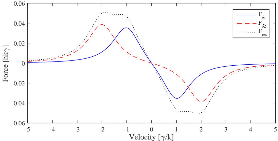
Figure 3.4: Force on the atom in 1D OM depending on its velocity. Previously calculated force with  $\delta_1 = \gamma$  is represented by the solid (blue) curve ( $F_{\delta_1}$ ). The force  $F_{\delta_2}$  corresponding to two counterpropagating laser beams with a detuning of  $\delta_2 = 2\gamma$  is shown by the dashed (red) curve. The addition of the two yields the dotted (black) curve for  $F_{res}$ .
