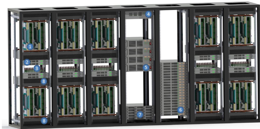
Figure 1.1: Rendered View of the NM-PM1 system. 1: Wafer Module, 2: Wafer Module network switch, 3: analog readout subsystem, 4: Top-of-Rack (ToR) 40 Gbit network switch, 5: storage server node, 6: computer server node, 7: Wafer Module power supply, 8: top and bottom fan units for Wafer Module. [8, p. 31]
