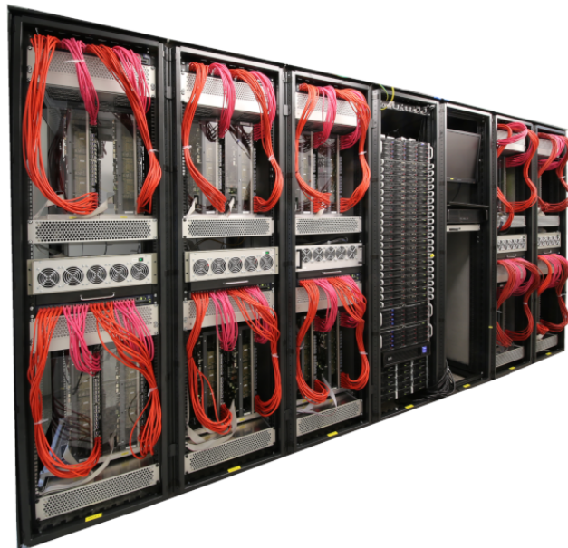
Figure 1.1: BrainScaleS neuromorphic compute system for 20 wafer modules. Each module has 384 HICANN chips with up to 512 neurons and 114 688 synapses each. This corresponds to 0.2 \times 10^6 neurons and 44 \times 10^6 synapses. For the complete system including 20 wafer modules in total this scales to roughly 3.9 \times 10^6 neurons and 880 \times 10^6 synapses.
