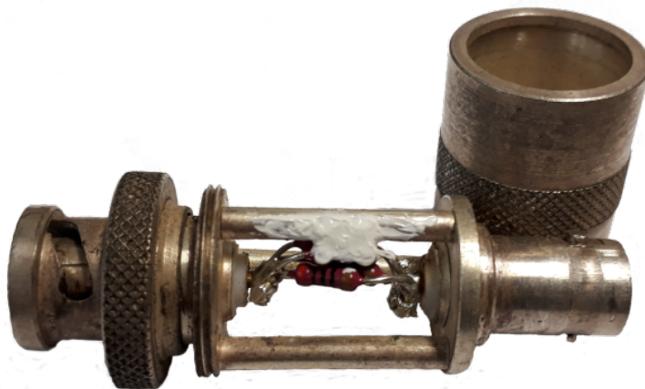
Figure 3.3: Series resistor adapter for buffering the SM output with 50 \Omega source impedance. Four 200 \Omega resistors have been soldered in between the inner conductor pins of the adapter. Heat-conductive paste has been used to offer heat exchange with the environment over the metal frame.
