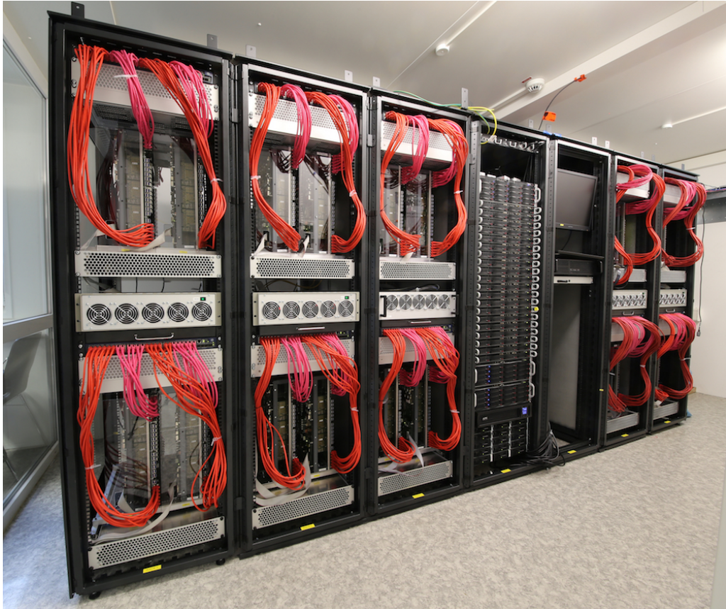
Figure 1: The BrainScaleS neuromorphic hardware including 20 wafer modules mounted in industry-standard racks. The red ethernet cables connect the modules to the host computer.
