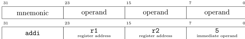
Figure 2.7.: Representation of Assembly Instruction addi as a Machine Instruction in Memory. The immediate value 5 is added to register r2 and the result written in r1 . Table A.1 shows a list of important instructions in the PowerISA.
