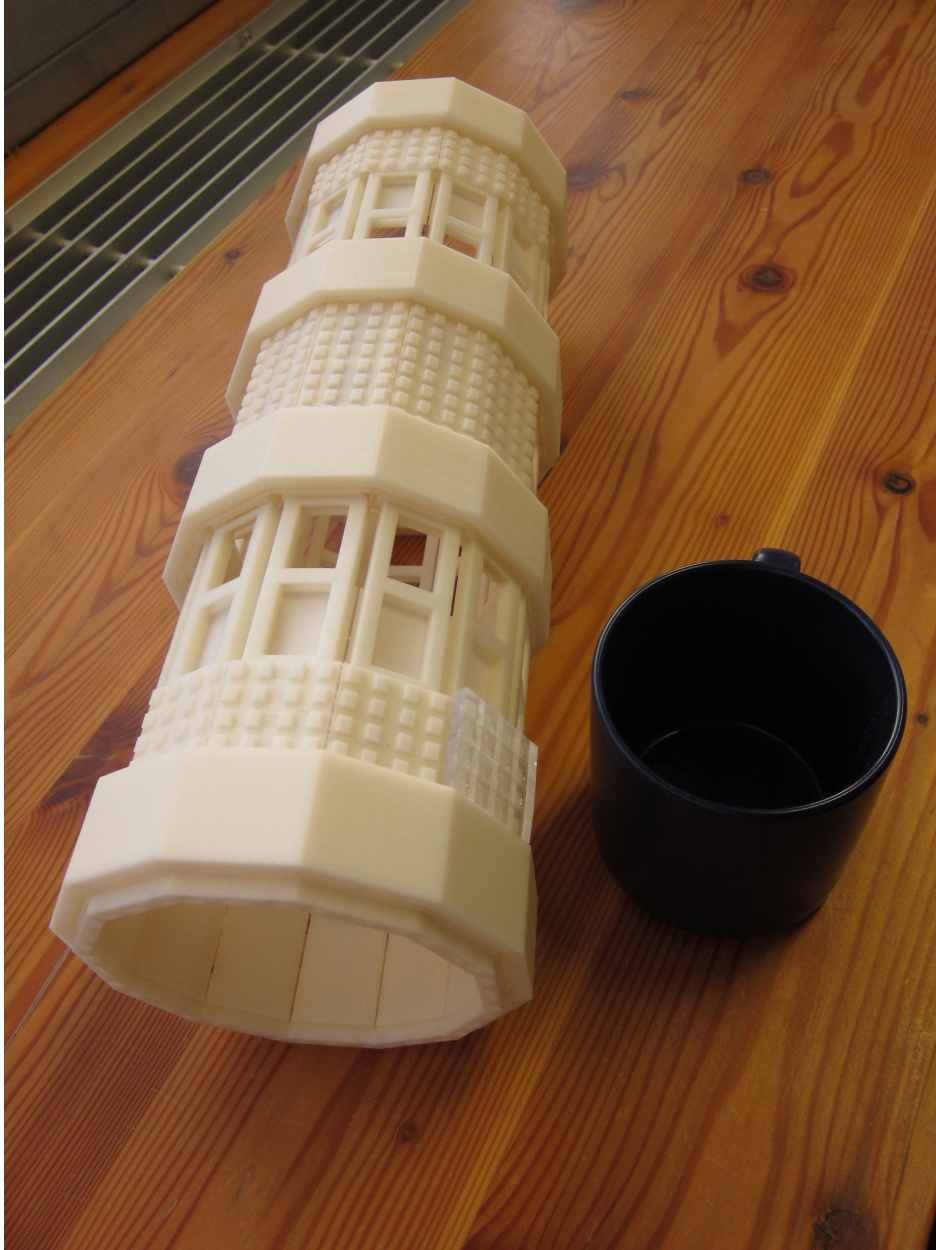
Figure A.3.: Tile Detector mockup based on an early 12-sided design. The tiles, SiPMs and readout boards are only partially shown.
