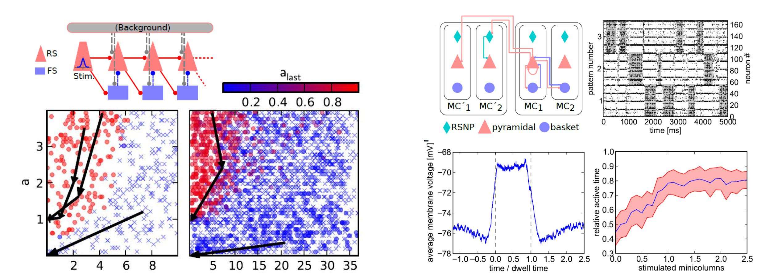
The configurability of the Spikey chip makes it a versatile general-purpose emulation device for spiking neural networks [8]. Left: Synfire chain network with feed-forward inhibition. Right: Cortical L2/3 attractor memory model.
