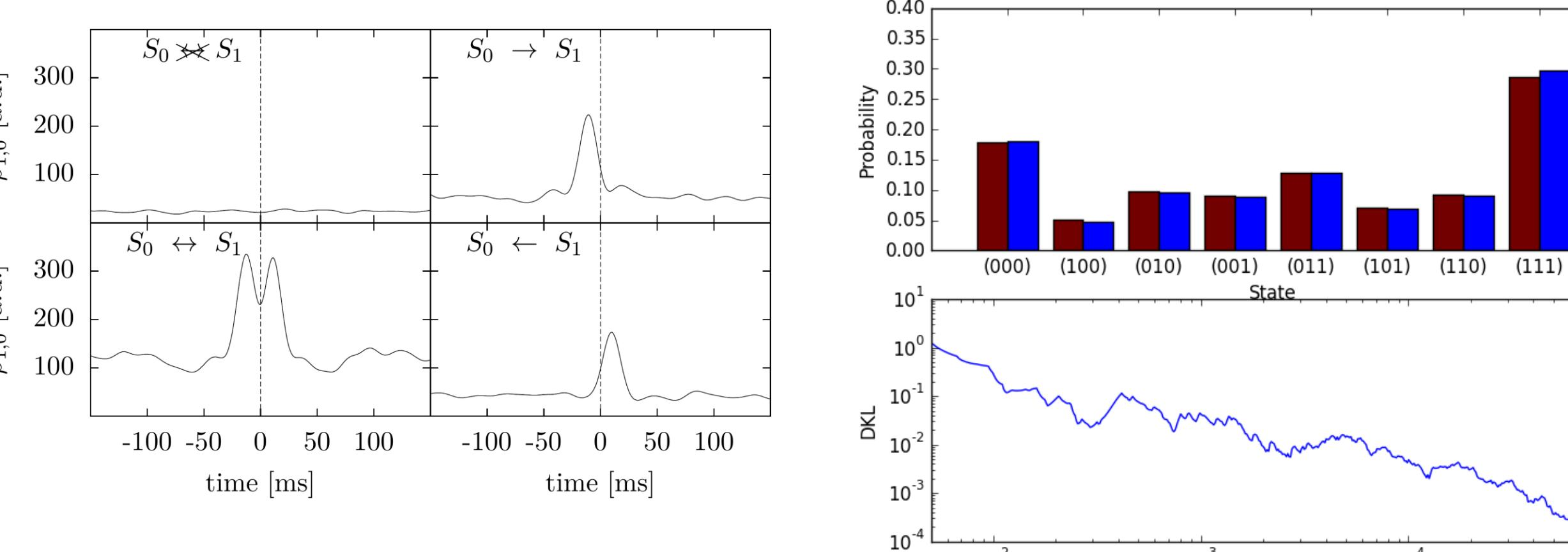
Left: Functional configuration of the lateral interaction between the sampling modules. Right: Sampling from a target distribution over 3 binary random variables on the Spikey chip. The entire experiment, with a duration of 100 s in biological time, takes only 10 ms on Spikey.
