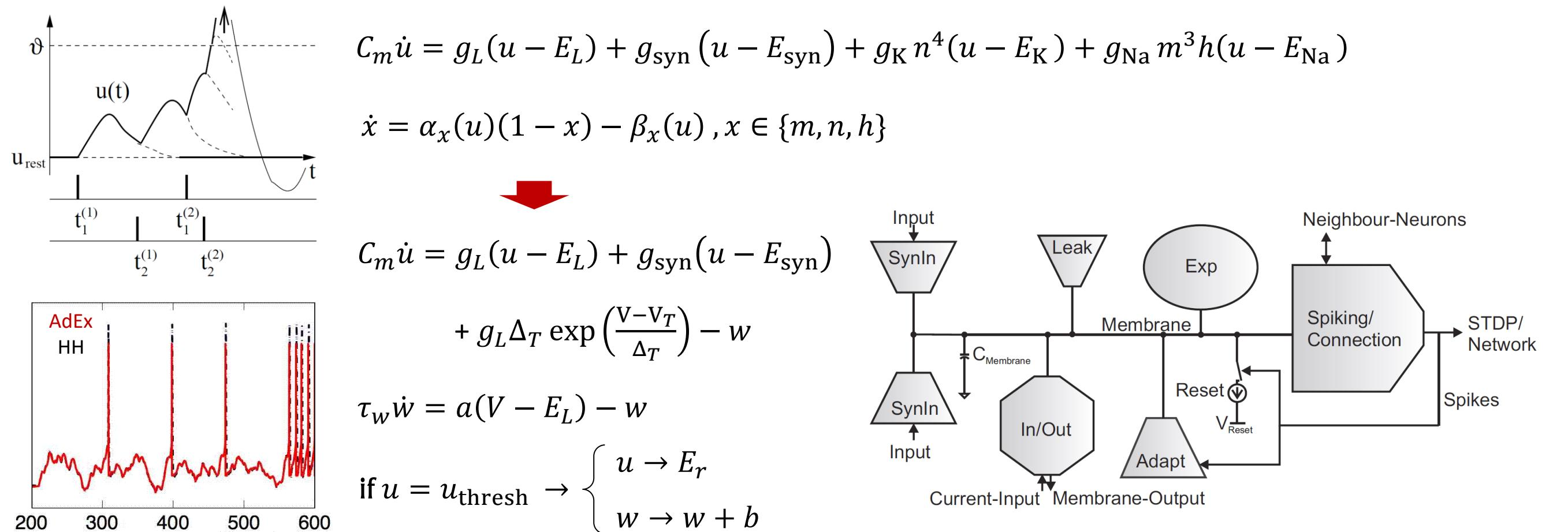
Left: Subthreshold and spiking dynamics of neuronal membranes. Middle: abstract models – Hodgkin-Huxley versus Adaptive Exponential Integrate-and-Fire (AdEx). Right: Embedding of model equations into VLSI circuits (schematic) [10].
