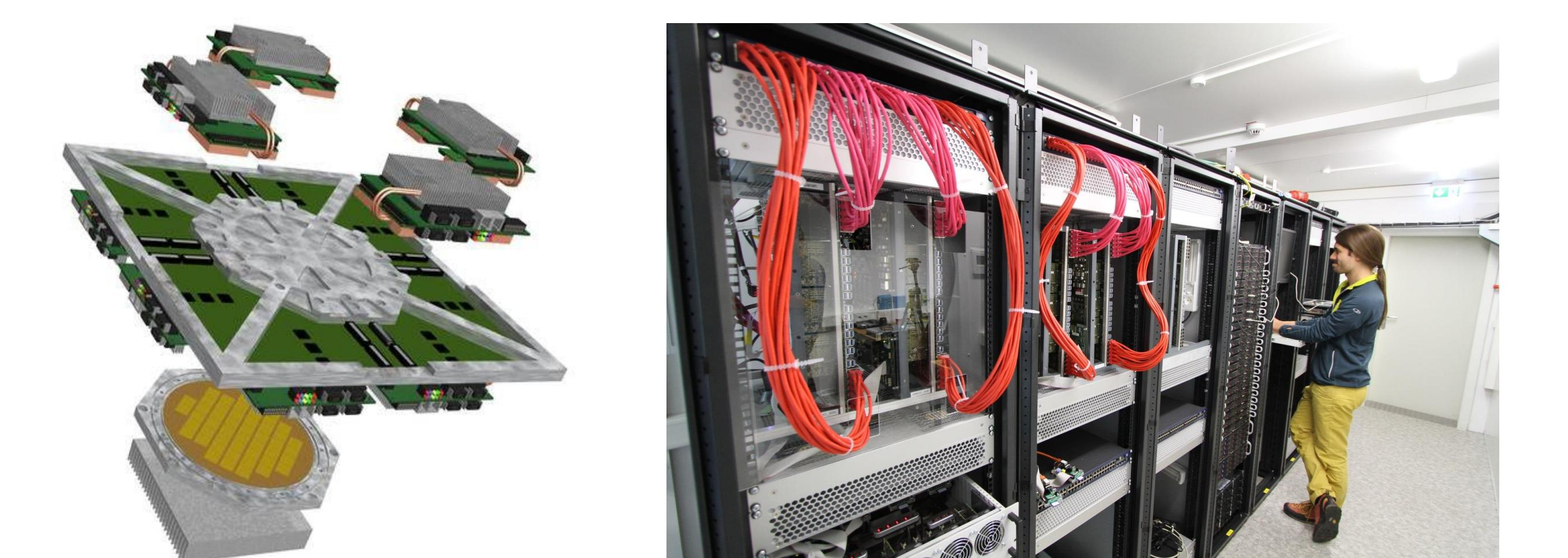
Left: Wafer-scale integration of 200k neurons and 50M synapses [10]. Right: Hybrid modeling facility.
