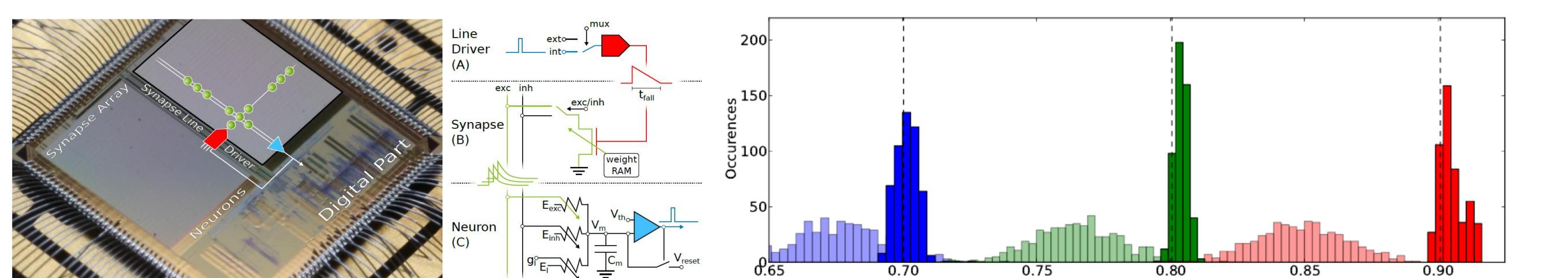
Left: Mixed-signal neuromorphic “Spikey” chip with highlighted communication infrastructure (384 neurons, 100k synapses) [8]. Right: Characterization and calibration of neuromorphic circuits (here, for the neuronal reset potential) [6,7].
