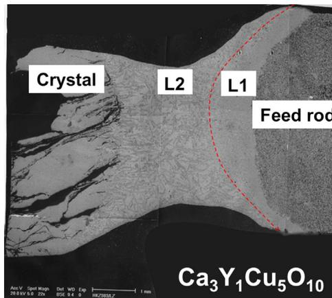
Fig. 3. SEM image of the quenched zone located between  $\text{Ca}_3\text{Y}_1\text{Cu}_5\text{O}_{10}$  crystal and feed rod. Liquid phase separation between the Y-rich melt  $L_1$  near the feed rod and Y-depleted melt  $L_2$  near the crystal is indicated.
