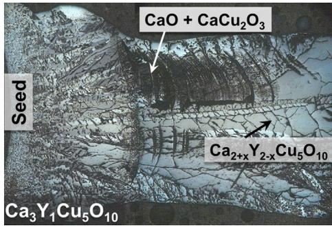
Fig. 2. Optical image in polarized light (longitudinal section) showing initial part of  $\text{Ca}_3\text{Y}_1\text{Cu}_5\text{O}_{10}$  crystal growth at 0.98 MPa oxygen pressure with  $v=0.38$  mm/h.
