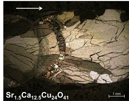
Fig. 1. Optical image in polarized light (longitudinal section) showing grain selection in initial state of  $Sr_{1.5}Ca_{12.5}Cu_{24}O_{41}$  crystal growth at 5 MPa oxygen high pressure with  $v=0.38$  mm/h. The arrow indicates the growth direction.
