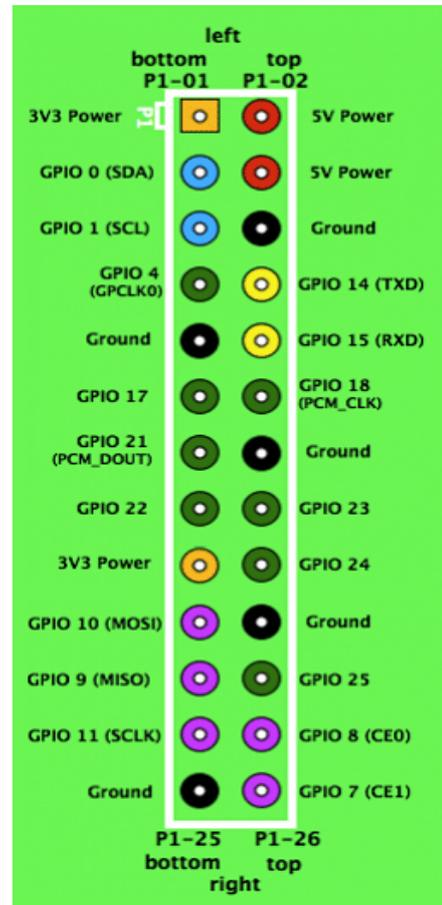
Figure 7: GPIO pin numbering on the Raspberry Pi P1 header [21].
