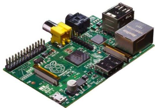
Figure 3: Raspberry Pi – size as big as a credit card. The header P1 is the one at the very left, equipped with pins. This header is used with the ribbon cable.
