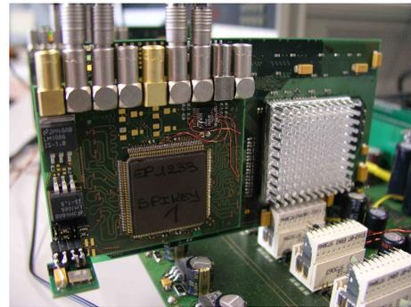
Fig. 1. A network module equipped with the VLSI ANN of [3] on the left.
