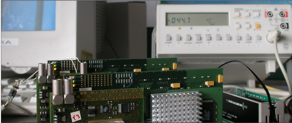
Figure IV.11: The experimental setup used for measuring the chip temperature.
