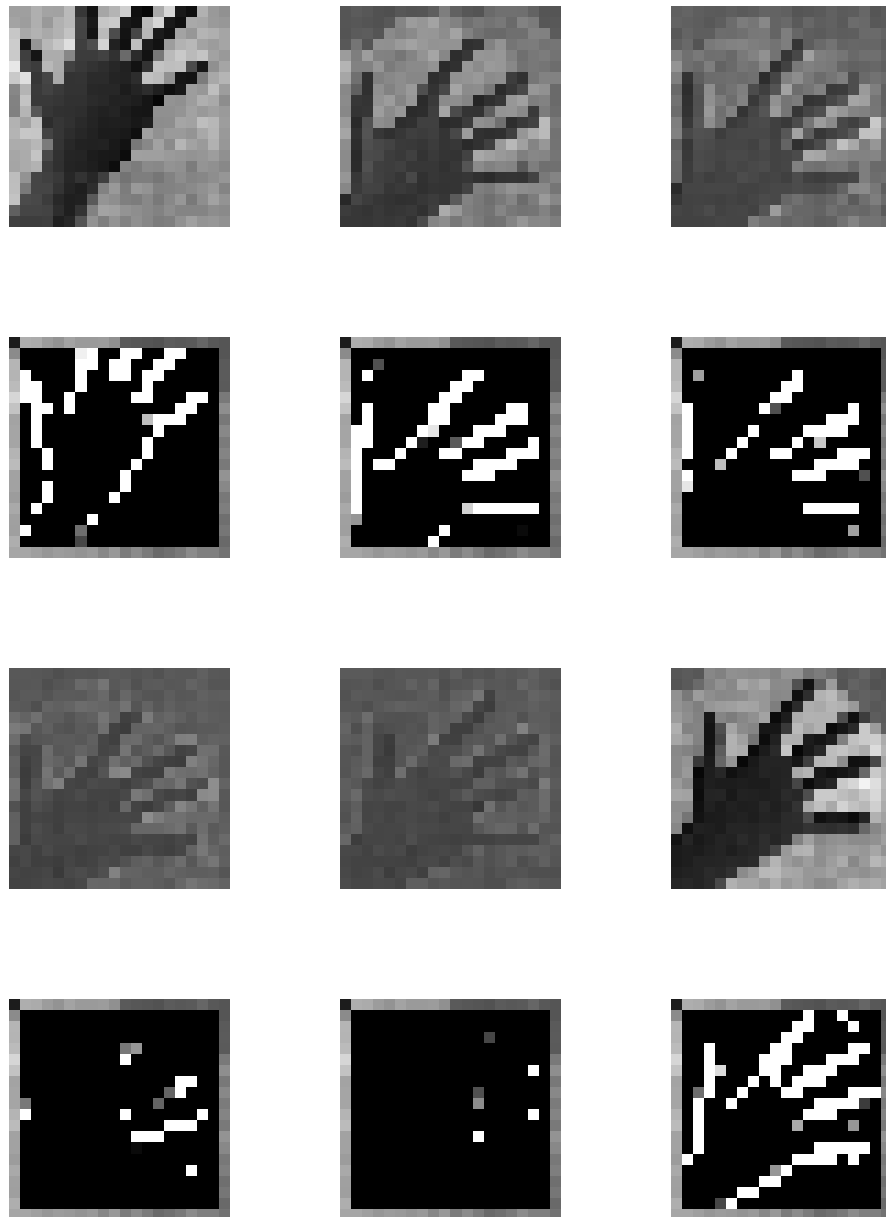
Figure 6: Simple moving object recorded with the 400 pixel adaptive camera. The first and the third row show a sequence of pictures recorded with the adaptive camera system. A hand is moving into the picture and held in position for a while. After pixel adaptation the hand is moved again and appears on the picture. The second and the fourth row show the output of a digital edge detection algorithm.
