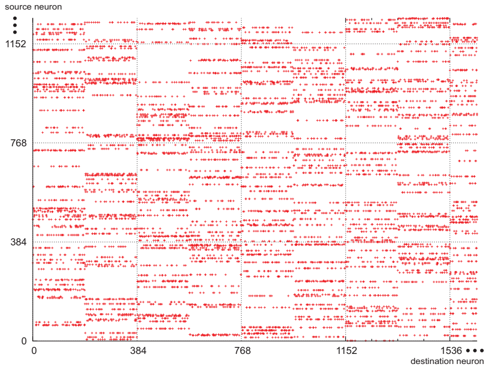
Figure 5.7: The neuron connectivity matrix of a 16-chip network with 10% synaptic efficiency. The reduction of the probability for the synapses to be activated increases the diversity or randomness of the generated networks. The resulting network load remains unaffected except for very low probabilities.
