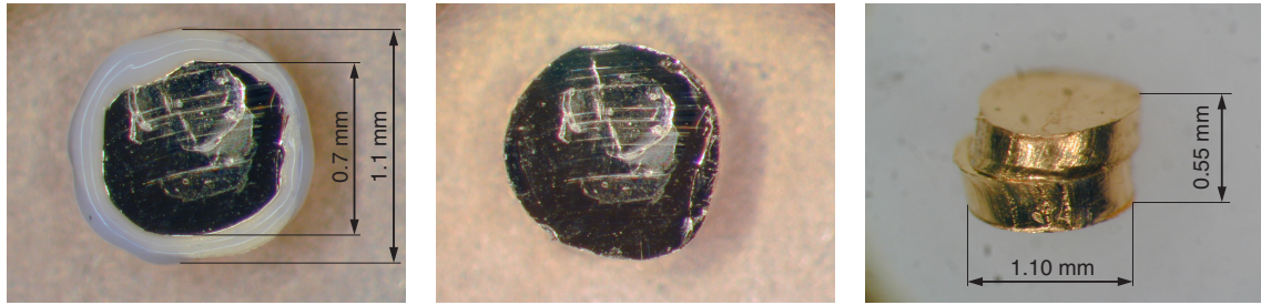
Figure 4.5 Left: The base area of one cylindrical disk is covered by a ring of polysiloxane. Inside the ring one can see the whitish ^{63}\text{NiCl}_2 crystals. Middle: The polysiloxane ring is removed. Right: The second cylindrical disk is pressed to the first disk encasing the source and both cylinders are diffusion-welded.
