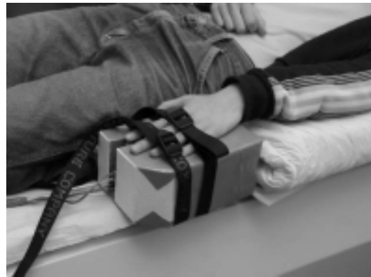
Figure 5.2: For tactile stimulation of the index finger, the module is inserted in a Styrofoam box.
