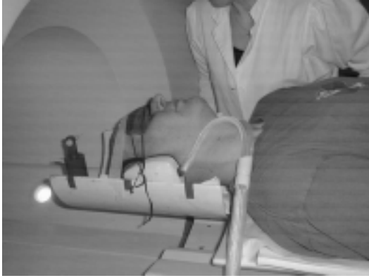
Figure 5.1: A blindfolded subject equipped with ear plugs and headphones. The head is taped to the head restraint.
