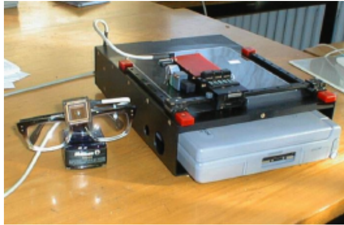
Figure 1 : Photograph of the VTD. The 3 rails and the tactile output unit are visible. The base unit is equipped with a laptop computer for control tasks. The photograph also shows a CMOS vision chip camera used together with the VTD to form a complete TVSS.
