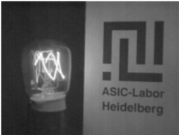
Figure 5.34: Image of a similar high dynamic range as seen in figure 5.33, taken with the logarithmic high resolution sensor Divichi.
