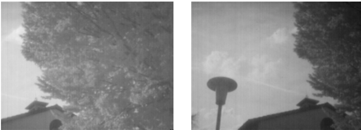
Figure 5.37: Example of the auto-exposure control. From left to right, the tree becomes darker since the mean intensity of the complete scene is increased.
